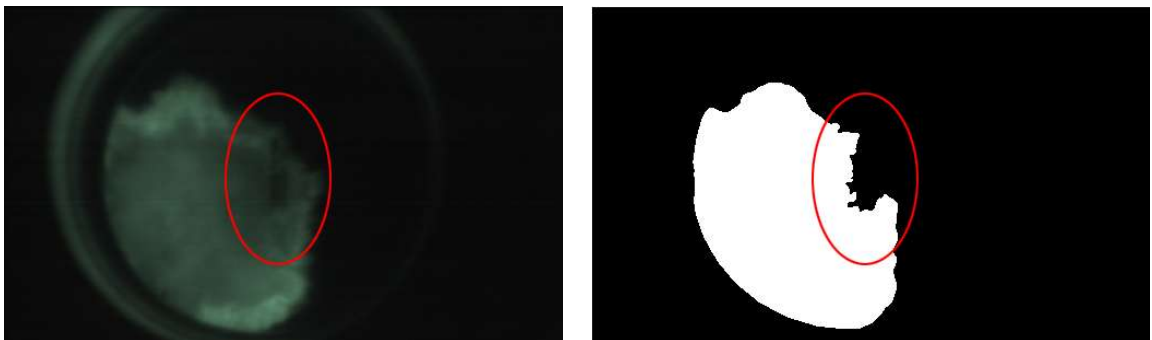
Figure 5.27 – Example of the issue involved with using the Otsu method of binarisation.
