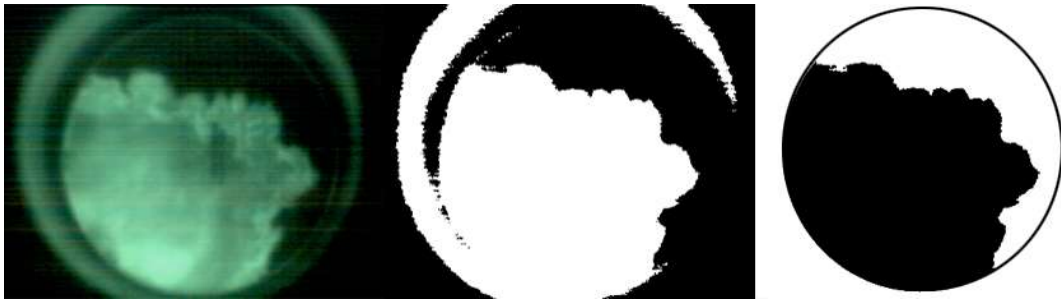
Figure 5.25 – Varying steps of image analysis shown together for the same initial image: Initial image taken with ICCD, mask-filtered binary image and the final inverted white-on-black arrangement (left to right).
