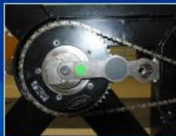
Figure 2. Instrumented crank arm (Axis Crank, Swift Performance, Aus).
