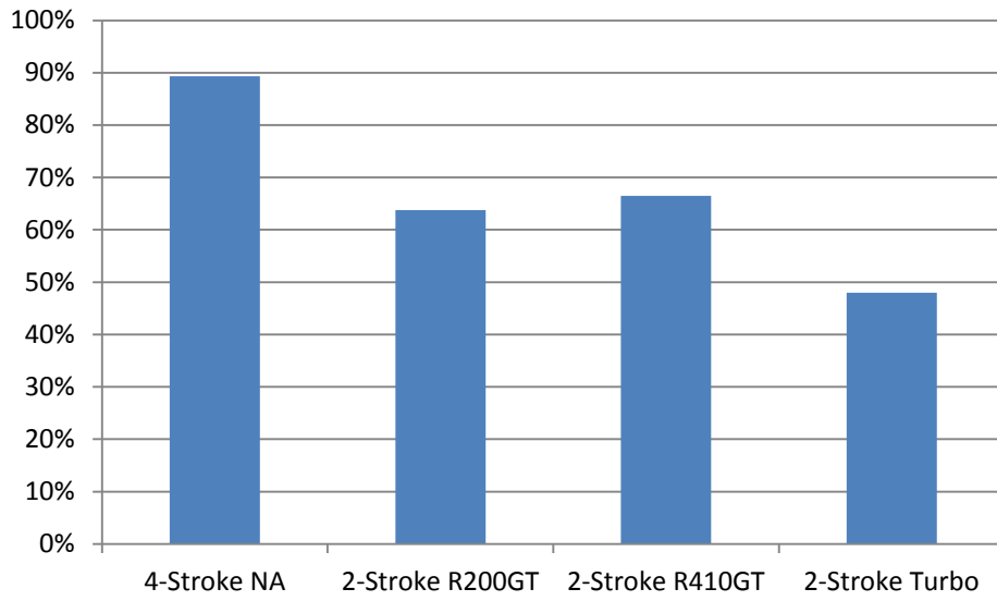
Figure 5.26 Charging efficiency at 4000rpm and 35kW
