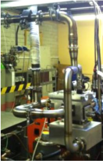
Figure 6.11 The intake(with blue pipes) and exhaust(wrapped by thermal isolation) layout in the single cylinder engine
