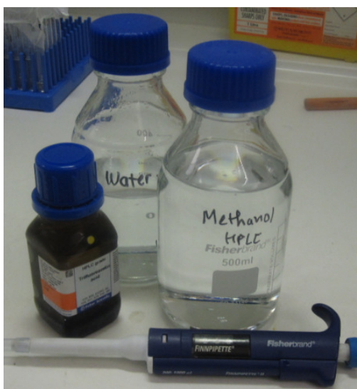
Figure 2.8 Methanol and water, to which 0.05% TFA was added for the HPLC mobile phase
