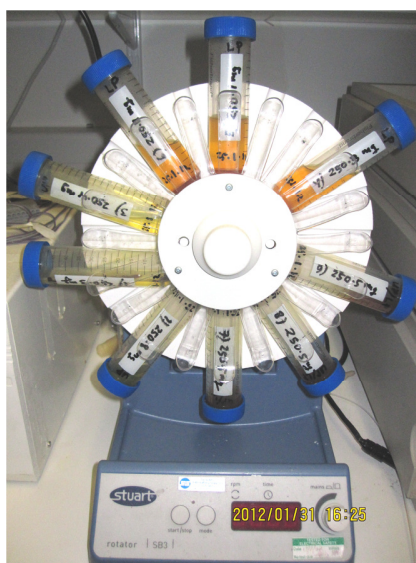
Figure 2.13 Extraction kinetic studies on a rotary wheel
