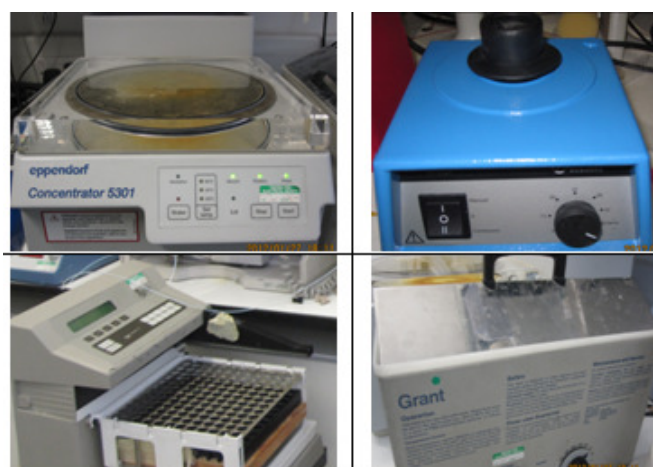
Figure 2.7 Supporting equipment e.g. (clockwise from top left) rotary concentrator, touch mixer, water bath and fraction collector
