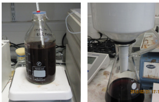
Figure 2.9 Preparation of aqueous ethanol extract with overnight maceration (left) and extract filtration under vacuum (right)
