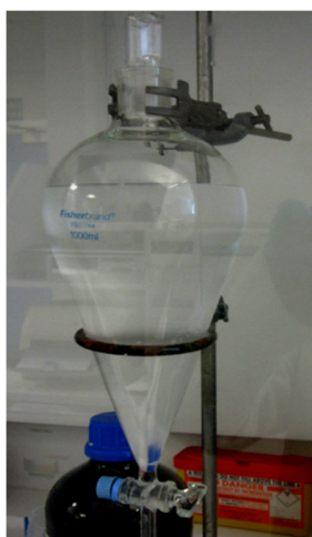
Figure 2.14 Solvent system preparations using a separating funnel
