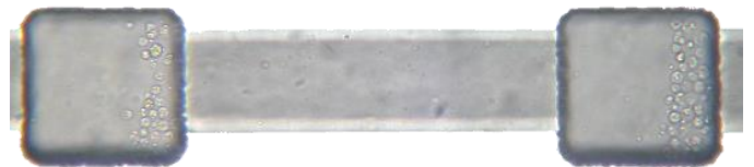
Fig. 2 Example of microscopy image of two subsequent chambers filled with CB MNCs. Cells were seeded at a flow rate of 0.2 \mu l/min.
