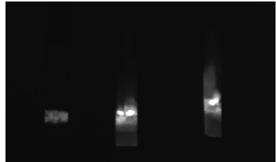
Figure 2.a: Chitosan modified test strips with 50mM DNA in pH 5.0 MES buffer bound to the test region
