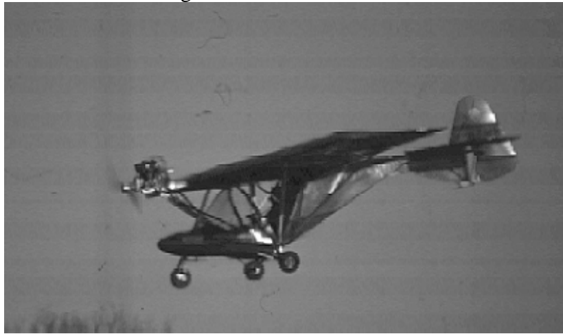
Light and draggy - the AX3, a typical microlight trainer
