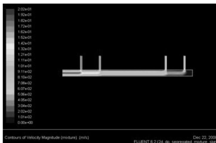
Figure 2.44 – Velocity distribution in common rail diesel component. (Li, et al., 2009)
