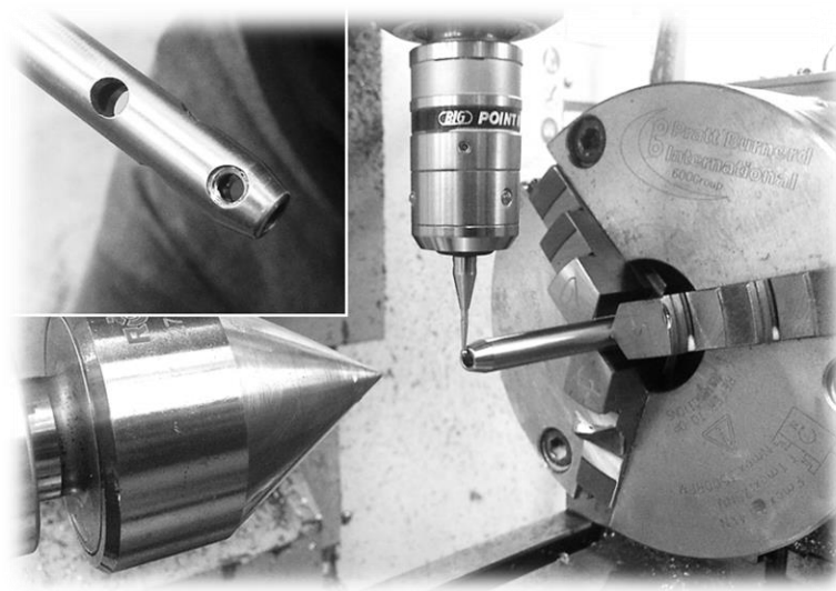
Figure 6.4 – Medical sample shaft for fatigue life testing following AFM.
