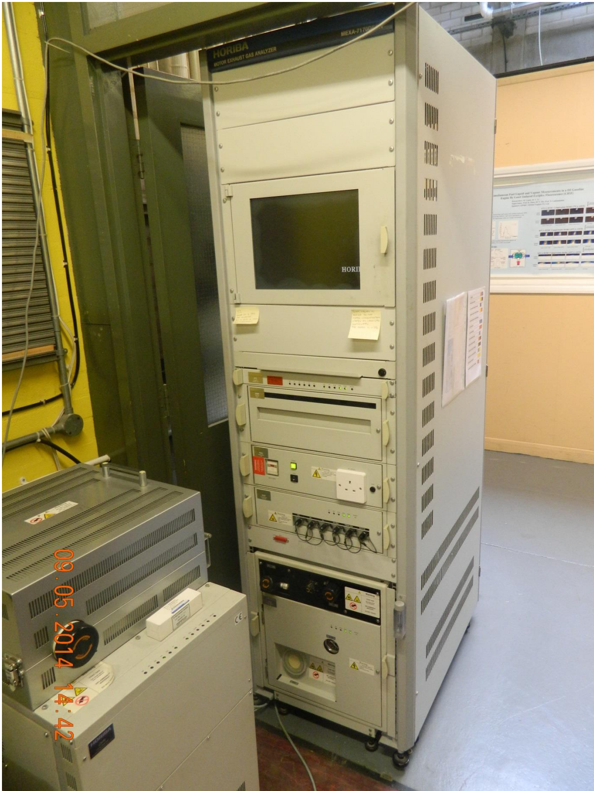
Figure (4.1): Horiba Mexa-7170 gas analyser.
