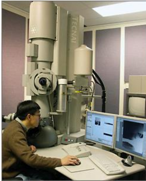
Figure (2.5): TEM microscope unit at National Renewable Energy Laboratory in USA.
