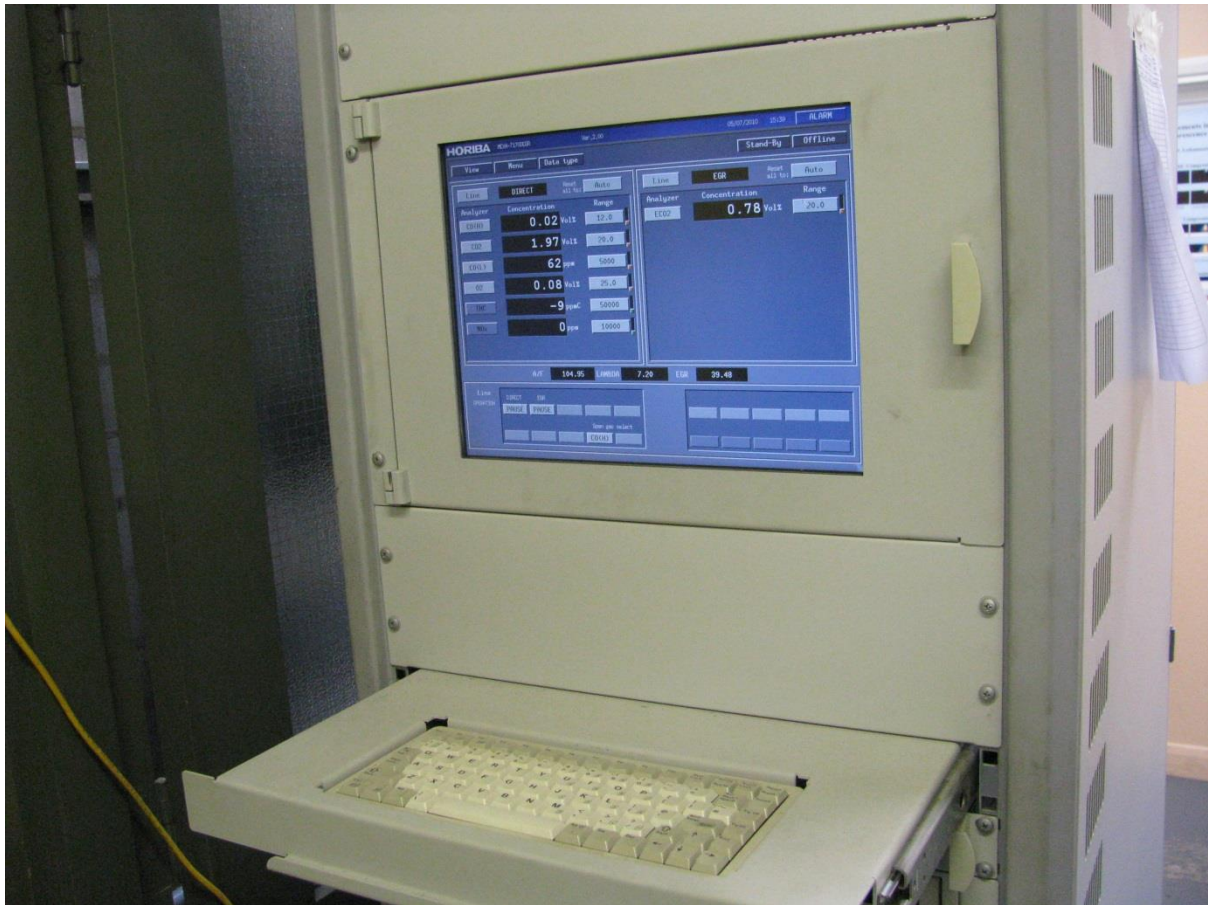
Figure (4.2): Horiba MEXA-7170 control system.
