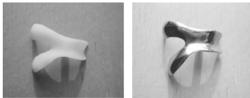
Figure 8.6: SL pattern of a hemi-knee joint (left), the titanium alloy joint (right) (He et al., 2006)
