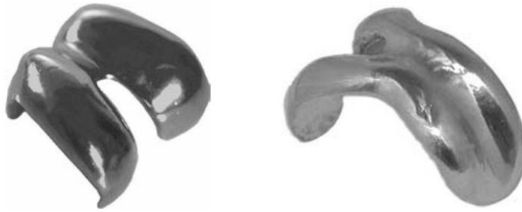
Figure 8.7: Custom- made femoral head by EBM a) Stainless steel b) Titanium alloy
