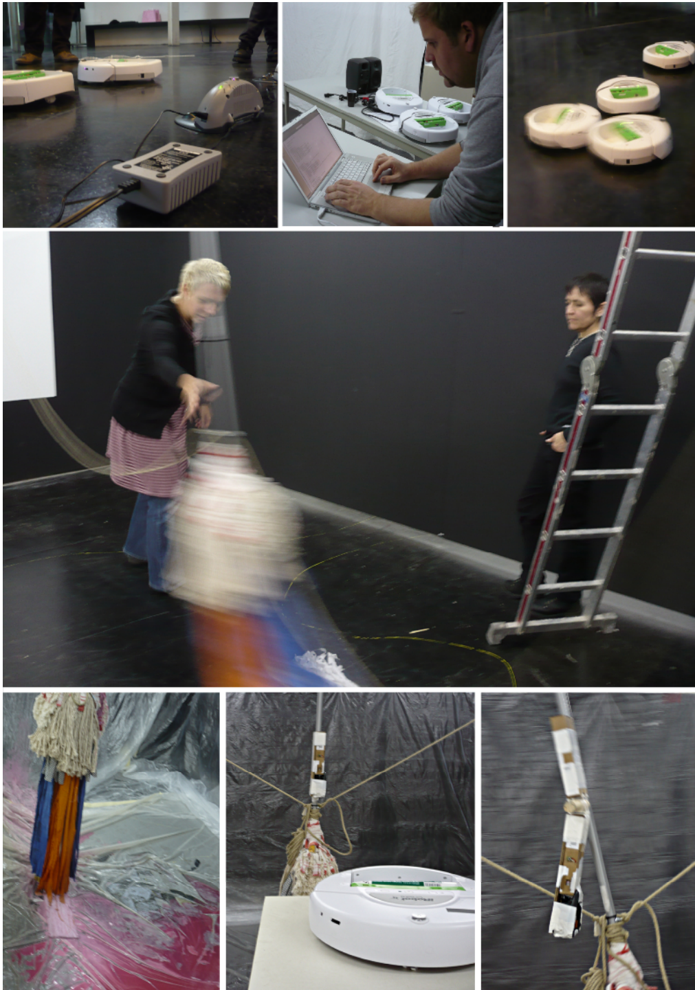
Fig.3.12: Prototyping of ON TRACK, in Vienna, February 2009. (a) First test with household robots ( iRobot Create ) (b) Rob Saunders programs the choreography of the robots (c) Four robots move and “dance” in sync (d) Petra Gemeinboeck and Linda Dement manually test the swing of the mop with a rope contraption (e) Fluids are distributed by the mop (f) The robots, placed on pedestals, are cued by the infrared signal attached to the passing mop (g) Mock-up detail of the infrared signaler. © in serial .
