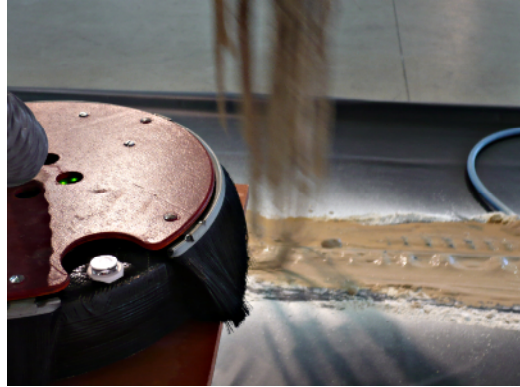
Fig. 3.5: Robotic brush with infrared sensor. © in serial .
