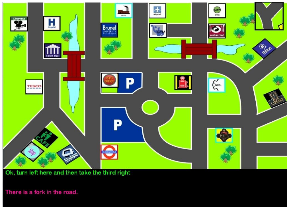
Figure 4.6. Screenshot of the user's interface during an interaction. The destination is the Tube station. The 'robot's' position is displayed in the small window on the top right of the user's interface. The dialogue box shows the user's message in green (on the top of the dialogue box) and the 'robot's' message in magenta (on the bottom of the dialogue box).
