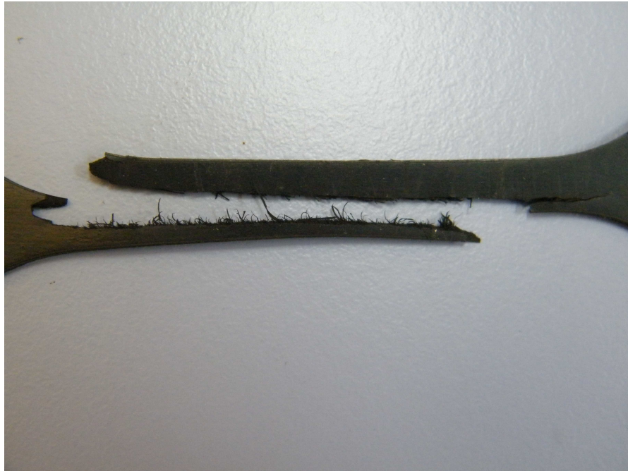
Figure 5.11: Typical fracture path for a low-crosslink-density rubber tested at a low applied strain rate ( \approx 5\%/min ): a) general b) close up of the fracture surface, please note the "hairy" appearance.
