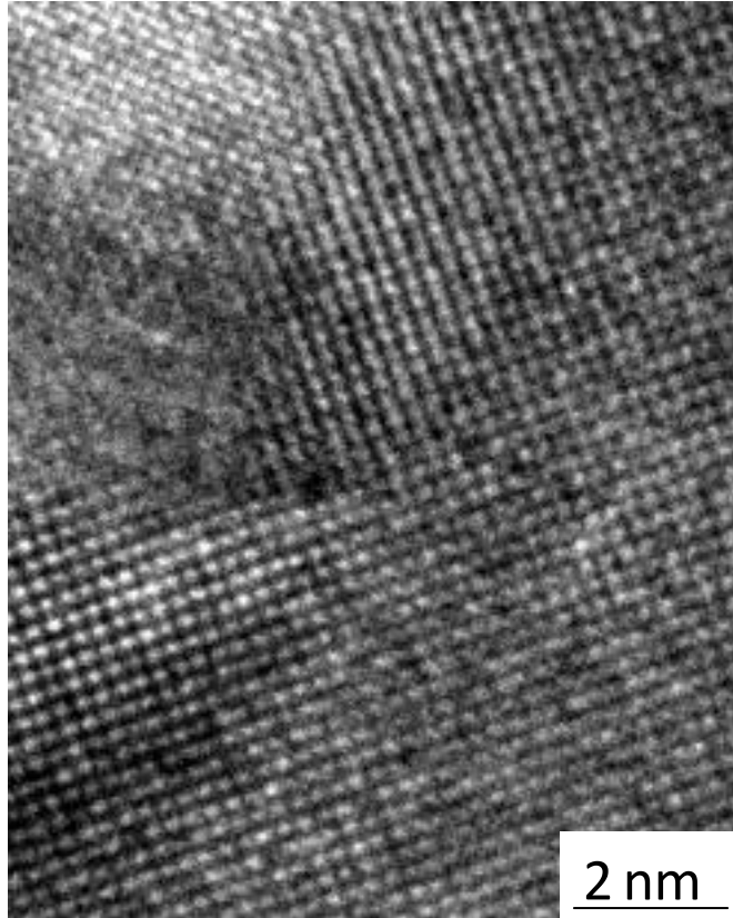
Figure 7.19 Precipitates of NbB 2 or Al 3 Nb phase with Al phase.
