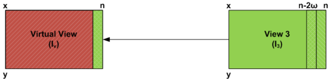
Figure 6.6: Extracting the relevant parts of view 3 to make the remaining part of the virtual view
