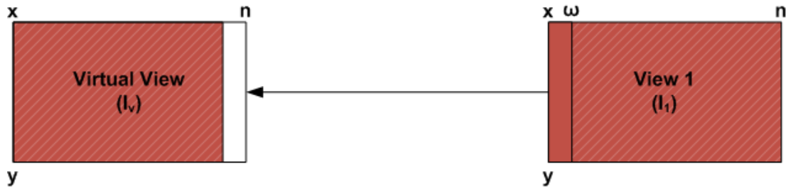
Figure 6.5: Extracting the relevant parts of view 1 to make the first part of the virtual view
