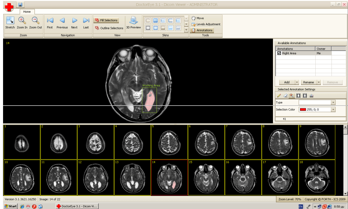
Figure 3.7: A single slide is selected for further processing. A working area has been set (green rectangle) and the segmentation algorithm has been applied. The selected area is labelled in pink.
