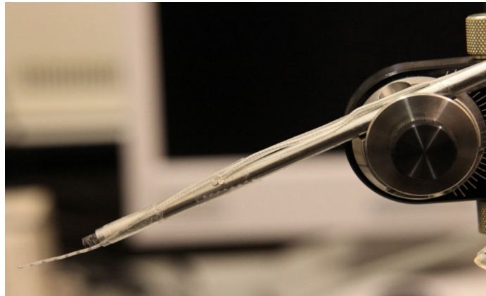
Figure 7.3-6. MED_EL cochlea electrode, taped to the micro positioning system
