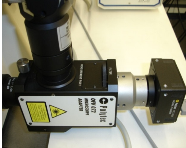
Figure 5.3-1. Beam splitter and microscope adapter connected to the microscope
