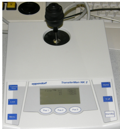
Figure 5.9-2, joystick and controller of the Eppendorf transformer
