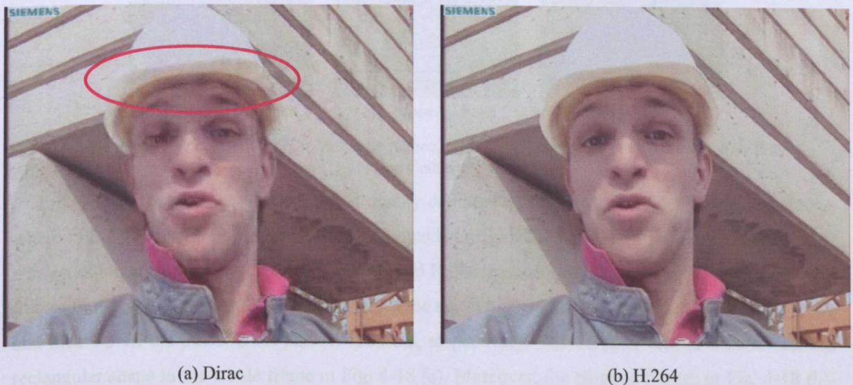
Fig. 4-17 Subjective Quality of Foreman Sequence in CIF Format (Frame Num. 83) with Inter Frame Coding, Target Rate 256 kbps
