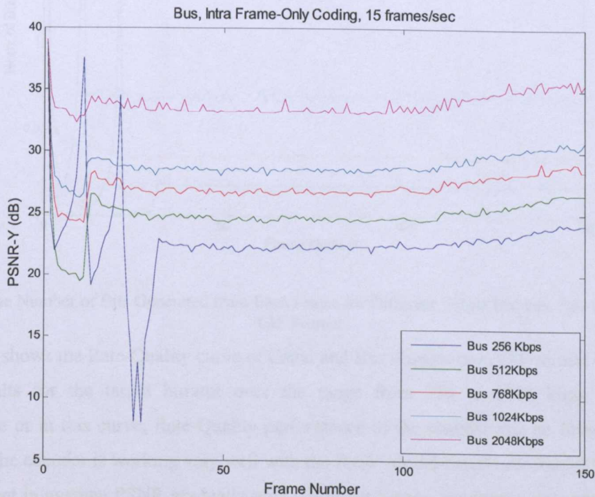
Fig. 4-7 PSNR Performance of Bus Sequence in CIF Format with Different Bitrates for Intra Frame-Only Coding
