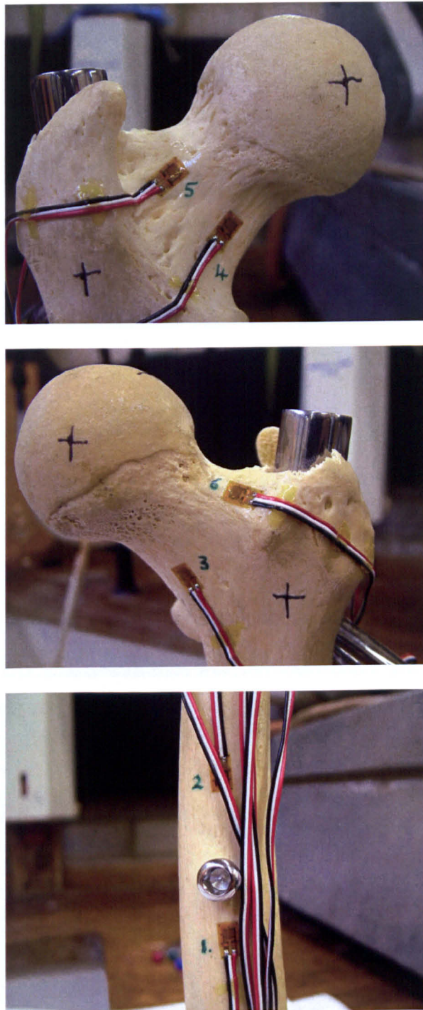
Figure 5.4 – Strain gauge positions on femur 2.
