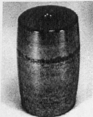
Figure 2.11 Surface distress in the form of a band encircling on a rolling element (SKF, 1994)
