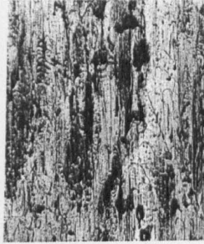
Figure 2.10 Smearing on a roller bearing surface from a spherical roller bearing – 100 x magnification (SKF, 1994)
