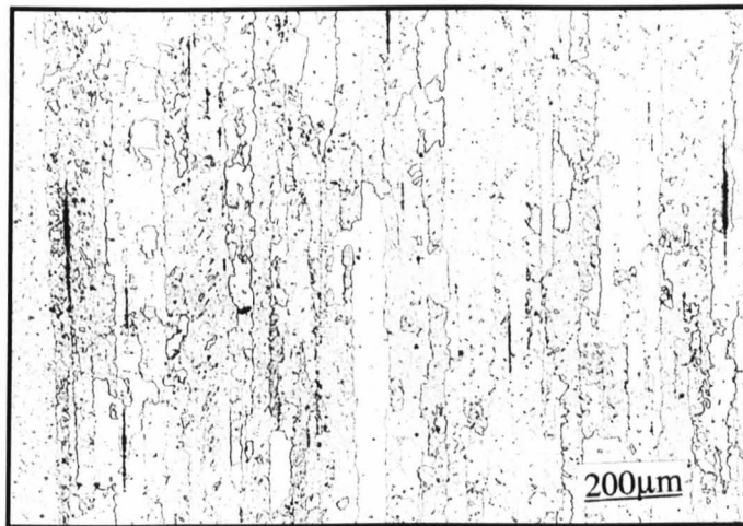
Figure 3-2 Microstructure of parent alloys in the recrystallized state (light micrograph).
