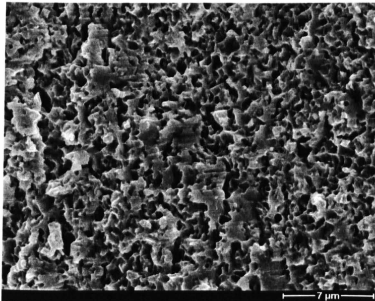
Figure 4-48 Fractograph of the shear test of the bonds made with the parent alloy in the recrystallized state at 1200 °C with a hold time of 30 minutes.
