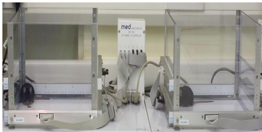
Fig. 3.3 Beam-breaker activity monitor chambers
