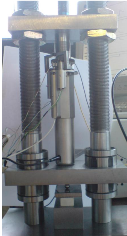
Figure 6.1 b) Image of device in test rig for static loading
