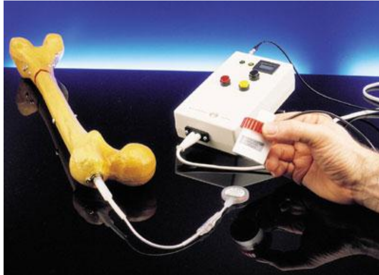
Figure 2-12 Fitbone -motorized distraction device (from Wittenstein Intens, 2008)
