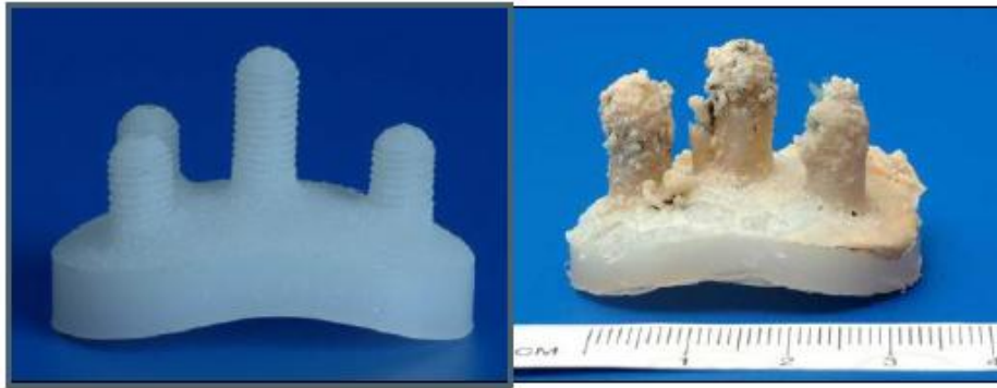
Figure 2-: Before implantation (left) & retrieved threaded implant (right) showing partially intact cement at the pegs (Yian et al. 2005).
