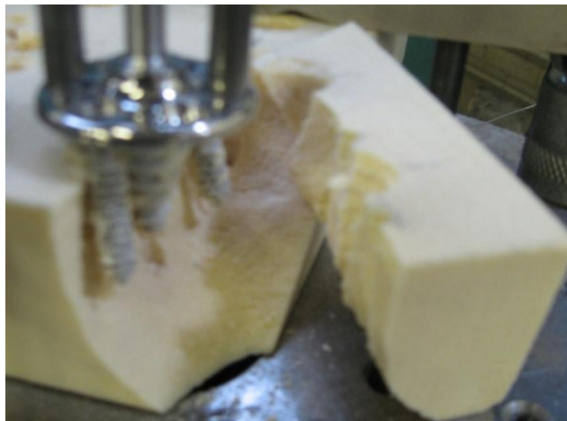
Figure 5-: GBP with 2 side screws tensile testing at 5mm/min
