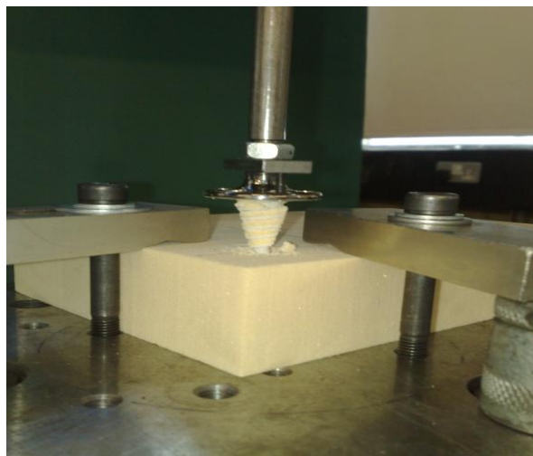
Figure 5-: Test (0) T1 GBP pulled out from the foam block
