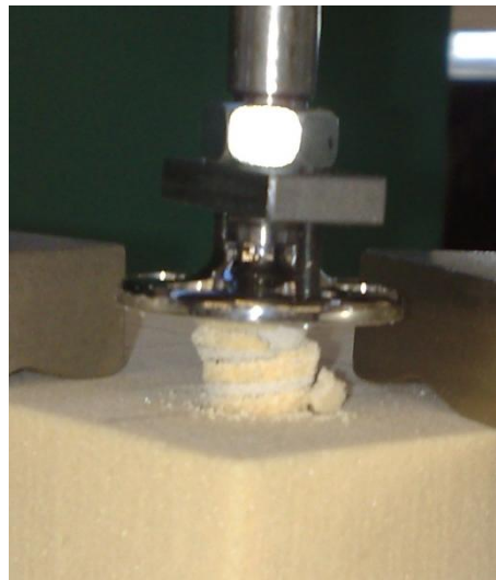
Figure 5-: Failure after cyclic and load to failure test in a with no side screw specimen
