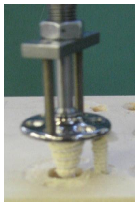
Figure 5-: T(1) T5(second repeat)GBP +1 side screw tensile testing
