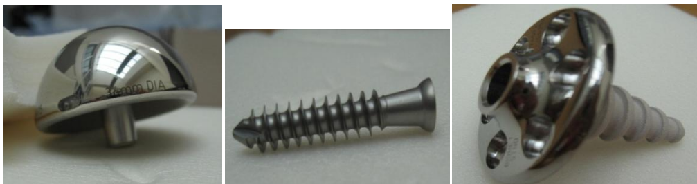
Figure 5-: The Implant parts used in the mechanical testing; Glenoid Head, Peripheral Screw and Glenoid Base Plate, respectively from left to right.
