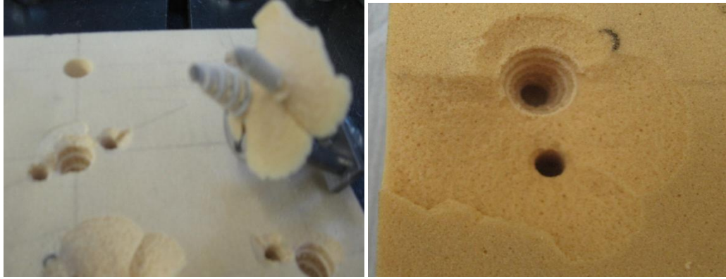
Figure 5-: GBP with +1 side screw after applying 20 mm/min failure loading
