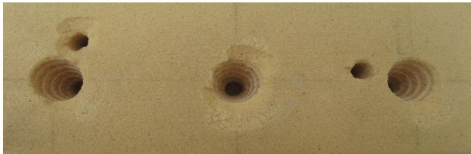
Figure 5-: GBP with 1 screw tensile testing at 5mm/min and 10mm/min
