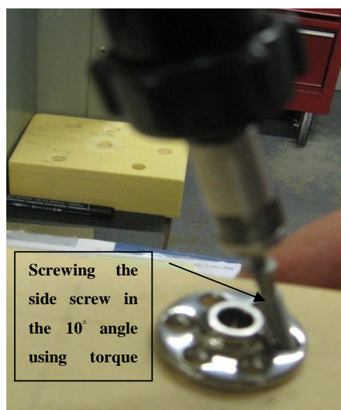
Figure 5-: Torque wrench used to screw the side screw in 10° angle
