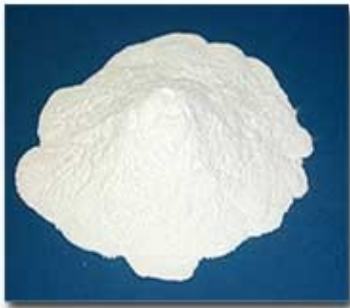
Fig. 2.7. Powdered PCM (Rubitherm GmbH, 2010)
