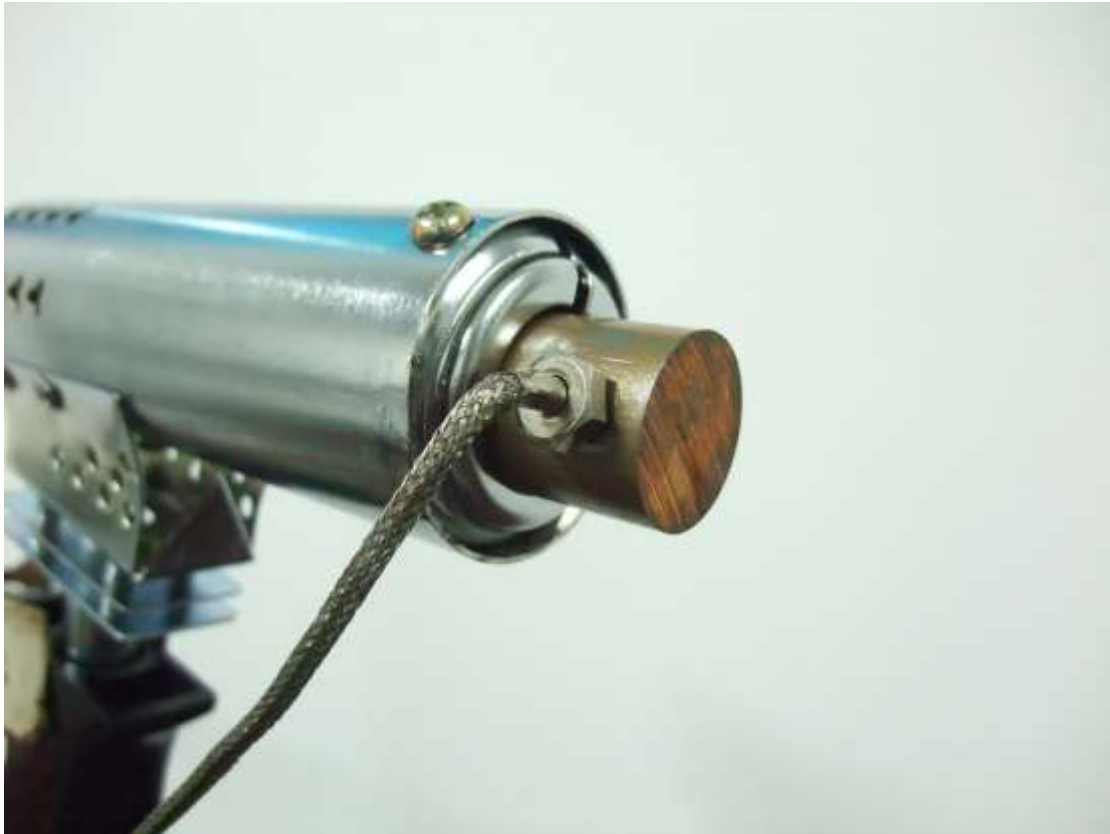
Figure 6.10b The touching point of a burn machine for making level 3 skin burn wounds
