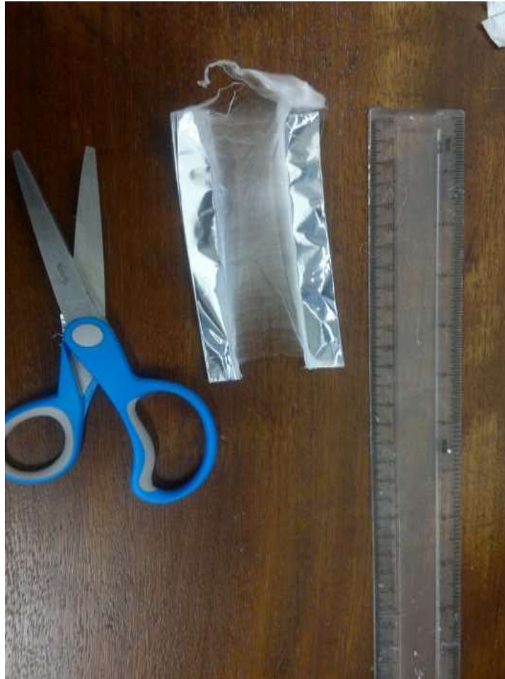
Figure 4.1 The fibre sheets were collected on two aluminum foil strips with some biased orientation across the gaps
