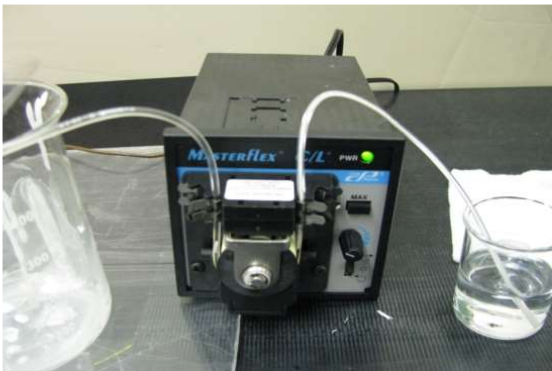
Figure3.5 Pump (Masterflex, 77120-52) with polymer solution
