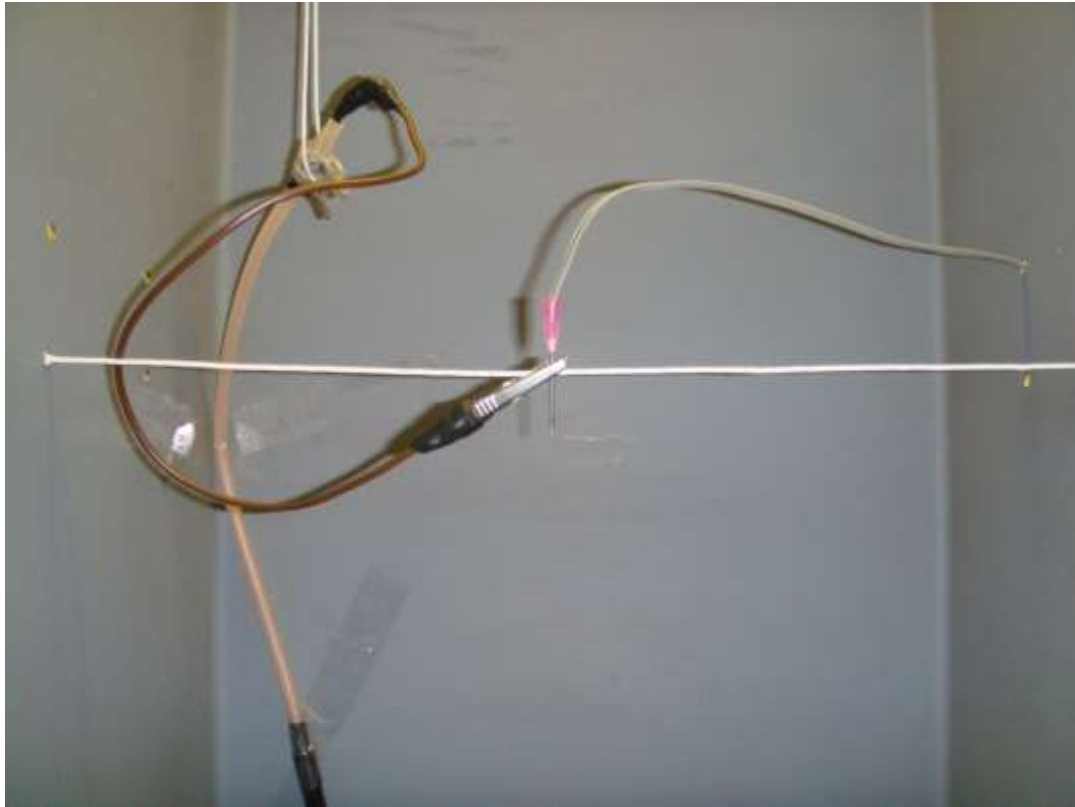
Figure 3.4 Needle with power supply and solution supply
