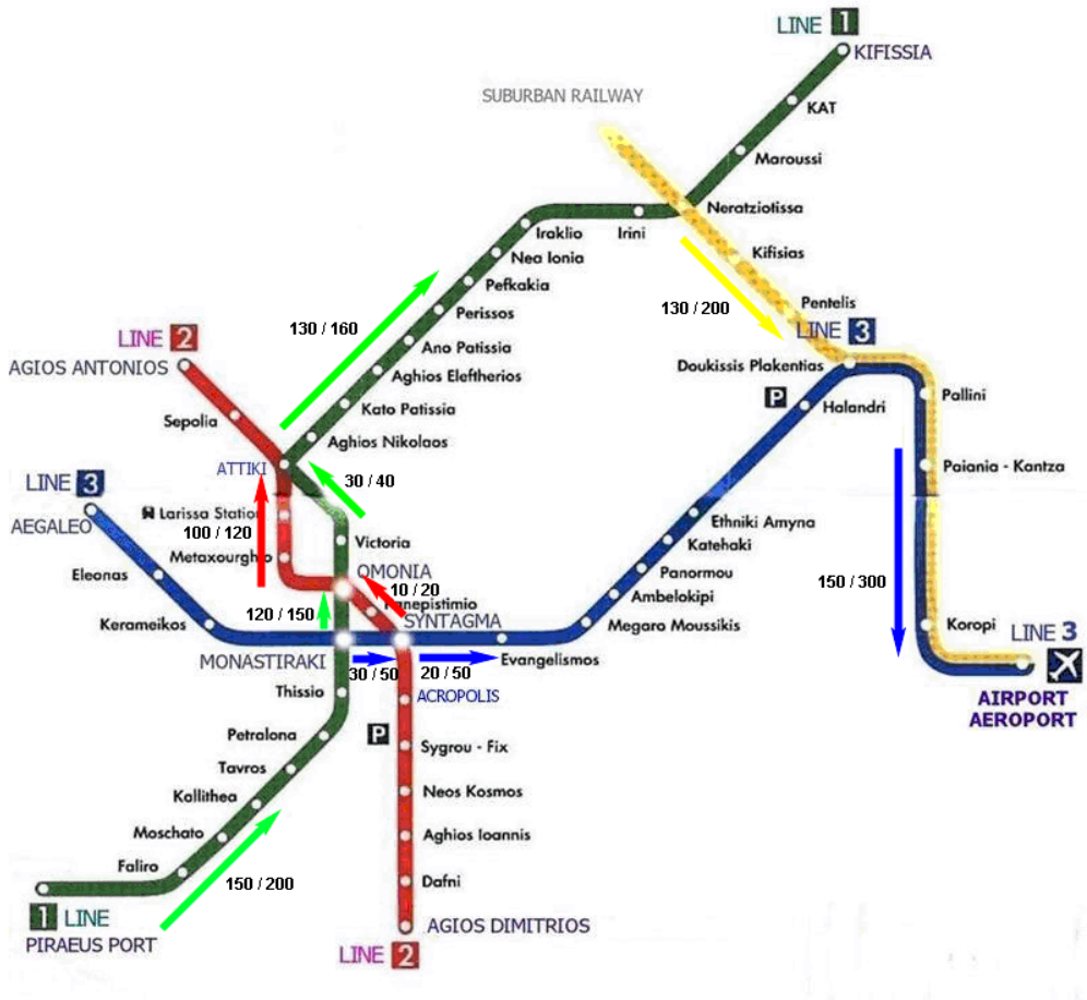
Figure 6-6 Metro lines as a flow network
