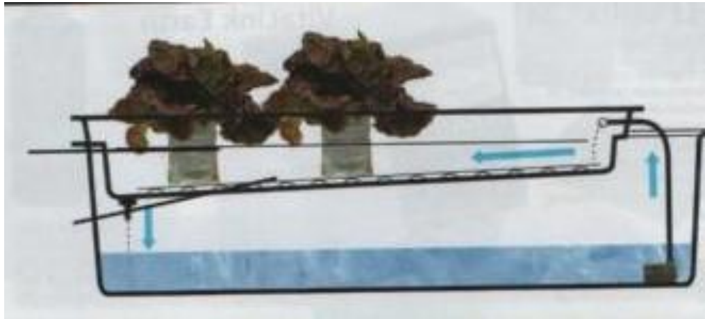
Figure 3.3 Working of a hydroponic culture system
