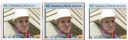
a. Pixel domain, frame 35 b. SL , 64kbit/s, Frame 35 c. s+q , 64kbit/s, Frame 35
