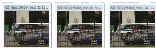
a. 75.27Kb/s, 23.96dB, Qp=46.08 b. 121.23Kb/s, 26.19dB, Qp=41.92 c. 193.58Kb/s, 28.52dB, Qp=37.76
