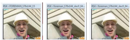
a. Pixel domain, frame 14 b. SL , 64kbit/s, Frame 14 c. t+s+q , 64kbit/s, Frame 14
