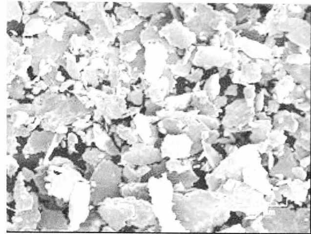
(b) Wear particles, B=0T , N=1 \times 10^6
