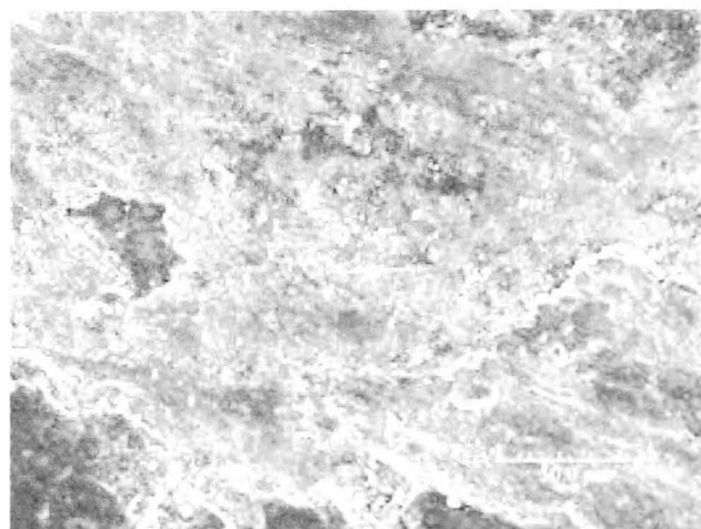
Rolling with Sliding, B=1.1T , N=1 \times 10^6
