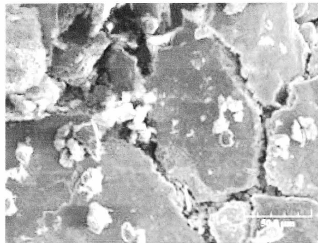
Rolling with Sliding, B=1.1T , \theta=90^\circ , N=5 \times 10^5
