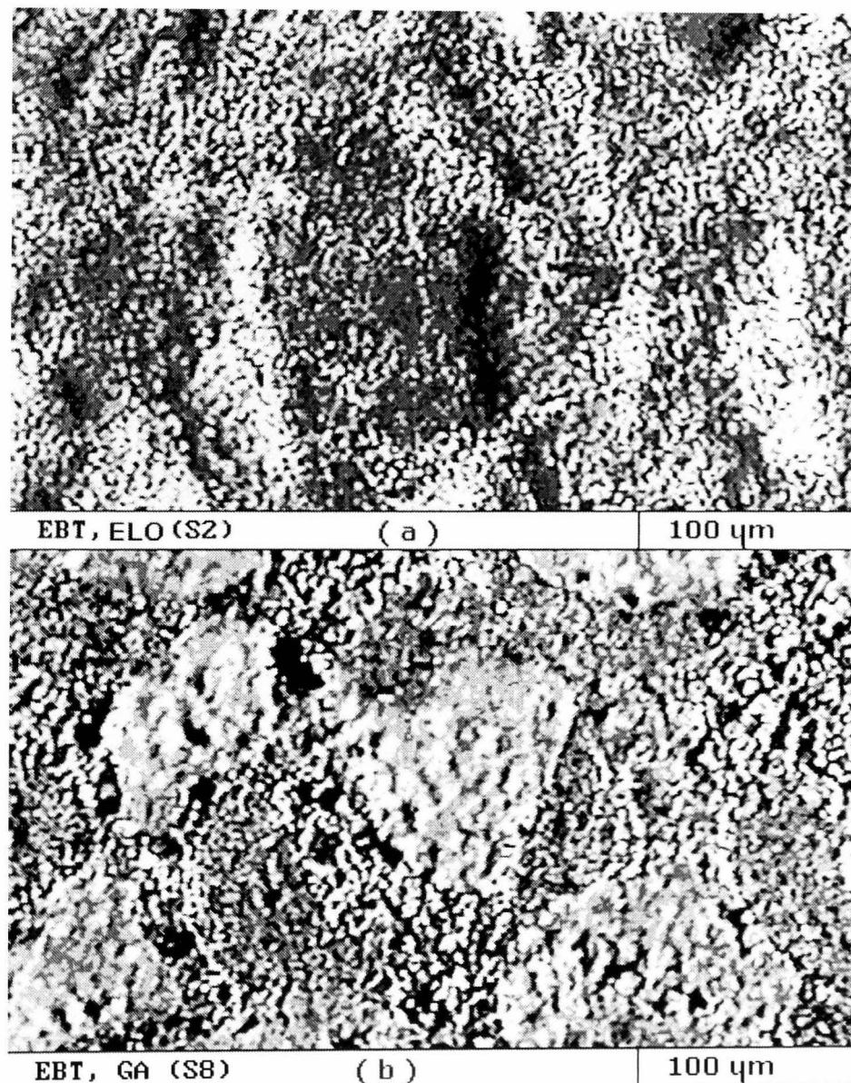
Figure 4.9 – Optical image of an EBT ELO coated (a) and GA coated (b) surface topographies
