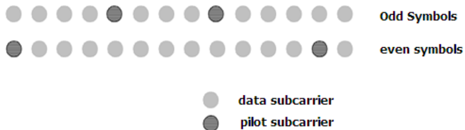
Figure 7: DL-PUSC Cluster Structure [1]
