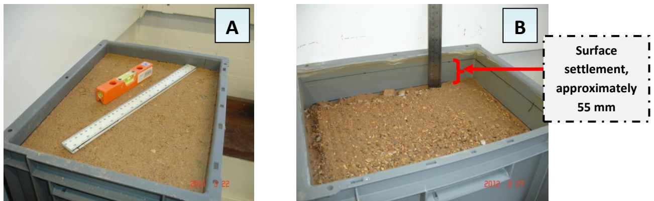
Fig. 4.92: Presents the box model experiment. Part A is for the model before 50 weeks of water flooding and part B is for the box after the 50 weeks (more details on this model work is in Section 3.9 of Chapter 3).
