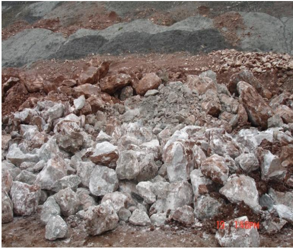
Fig. 1.7: Bantycok Gypsum- (Nottinghamshire/UK), the general size of collected blocks is 45 cm x 45 cm x 55 cm.
