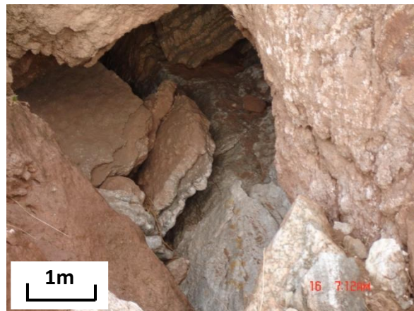
Fig. 2.5: Karstic features in gypsum rock. Sinkhole formed in gypsum rock at Bazyan, Iraq.
