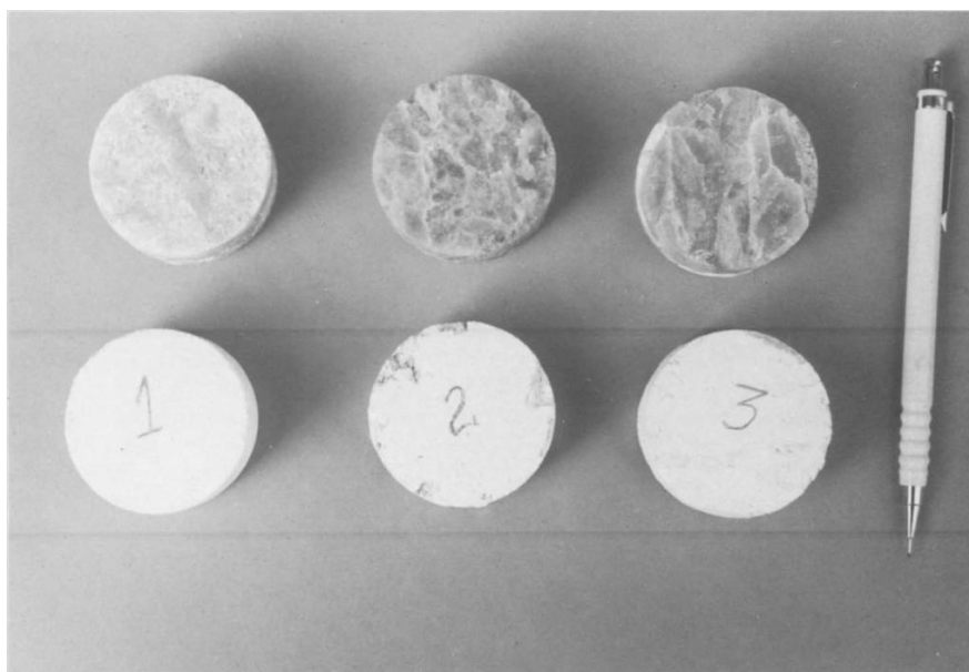
Fig. 2.9: Gypsum rock discs in 50 mm diameter tested; (1) alabaster, (2) medium-sized crystals, (3) coarse-sized crystals (from Papadopoulos et al., 1994, Figure 1). (Note: the samples size and shape are very similar to the thin-layer samples of this research).
