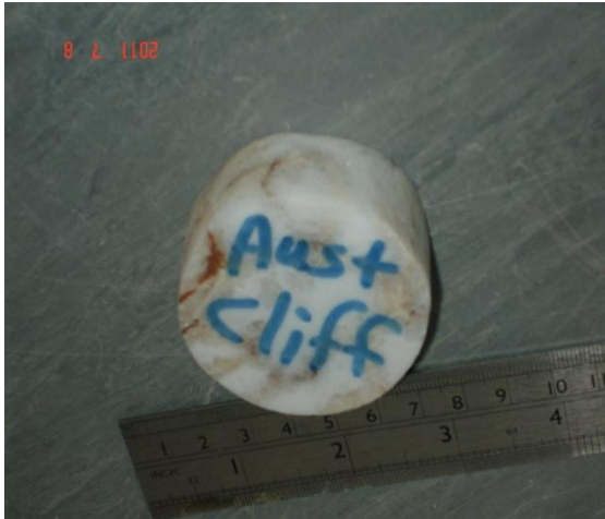
Fig. 3.36: Aust Cliff thin layer/discs sample, diameter is 54 mm and height is 20 mm. This sample was used for short-term compression testing.
