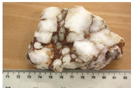
Fig. 2.2: Gypsum block from Aust Cliff collected on November 2009. See the existing cracks fill with particulate sediment minerals.
