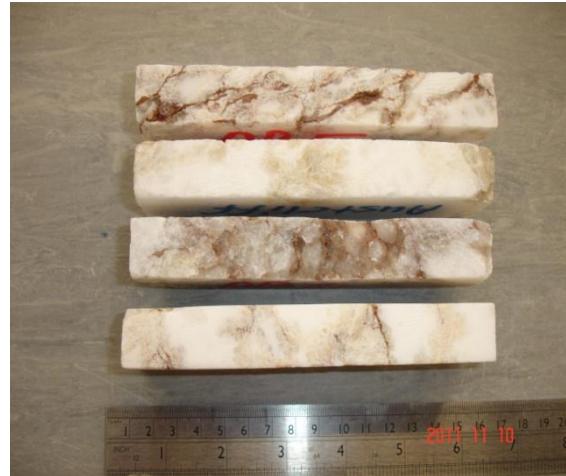
Fig. 3.37: Aust Cliff four-point bending samples, each bar size is 140 x 40 x 20 mm. These bars were used in short-term bending test.
