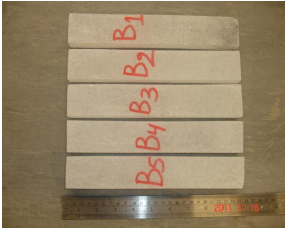
Fig. 3.40: White four-point bending bars, large size of 240 x 40 x 20 mm, from Bantycok samples, UK. These bars were used for short and long-term bending tests.
