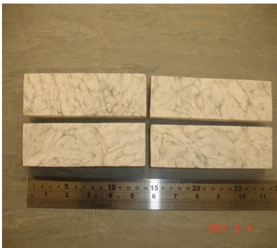
Fig. 3.34: Iraqi gypsum rock bars, used for four-point bending experiment, small size of 140 x 40 x 20 mm. These samples were used for short-term bending test.
