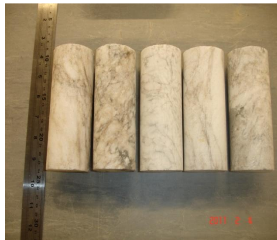
Fig. 3.35: Iraqi gypsum rock cylindrical samples: diameter is 54 mm and L/D is 2.5. These samples were used for short and long-term compression tests.
