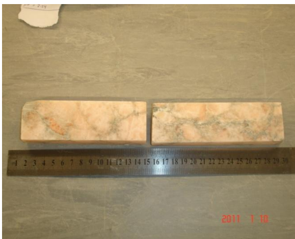
Fig. 3.38: Pink four-point bending bars, from Bantycok samples, UK, (each bar size is 140 x 40 x 20 mm). These bars were used for short-term bending test. Samples numbers are P1 and P2.
