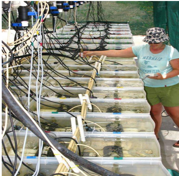
Figure 2.4. Photograph of the outdoor aquarium at Lizard Island where tanks are supplied with fresh seawater pumped directly from the lagoon.
