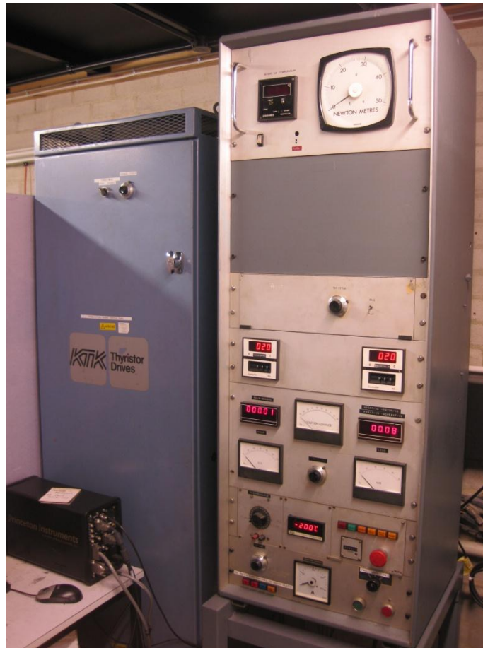
Figure 3.11 Left: KTK thyristor convertor unit; Right: Hydra control console
