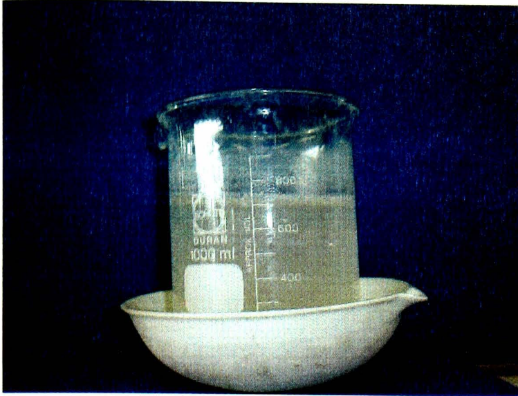
Figure-2.12 (a) Salt water collected after the 1 st series of countercurrent leaching process
