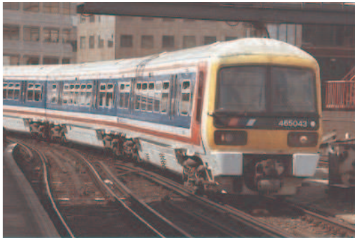
Figure 2.5.3 – Class 465 750 V DC traction unit at Waterloo East
