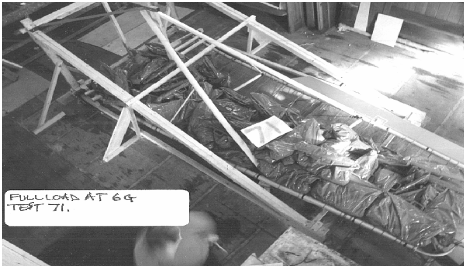
Figure 5 - Load Testing of a Wing (Raj Hamsa X' Air Mainplane, 6g, sail removed)
