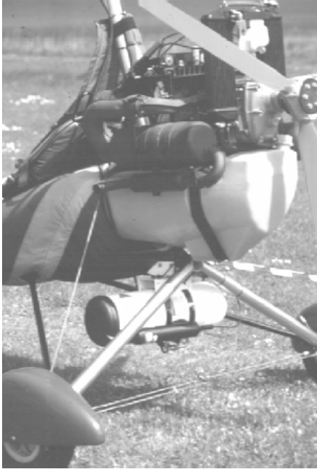
Figure 10 - BRS recover parachute fitted beneath Pegasus trike
