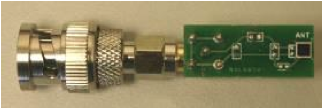
Figure 6.5: The full PCB with, mounted micro antenna to the right, impedance matching network in the centre, and the BNC connector to the left.
