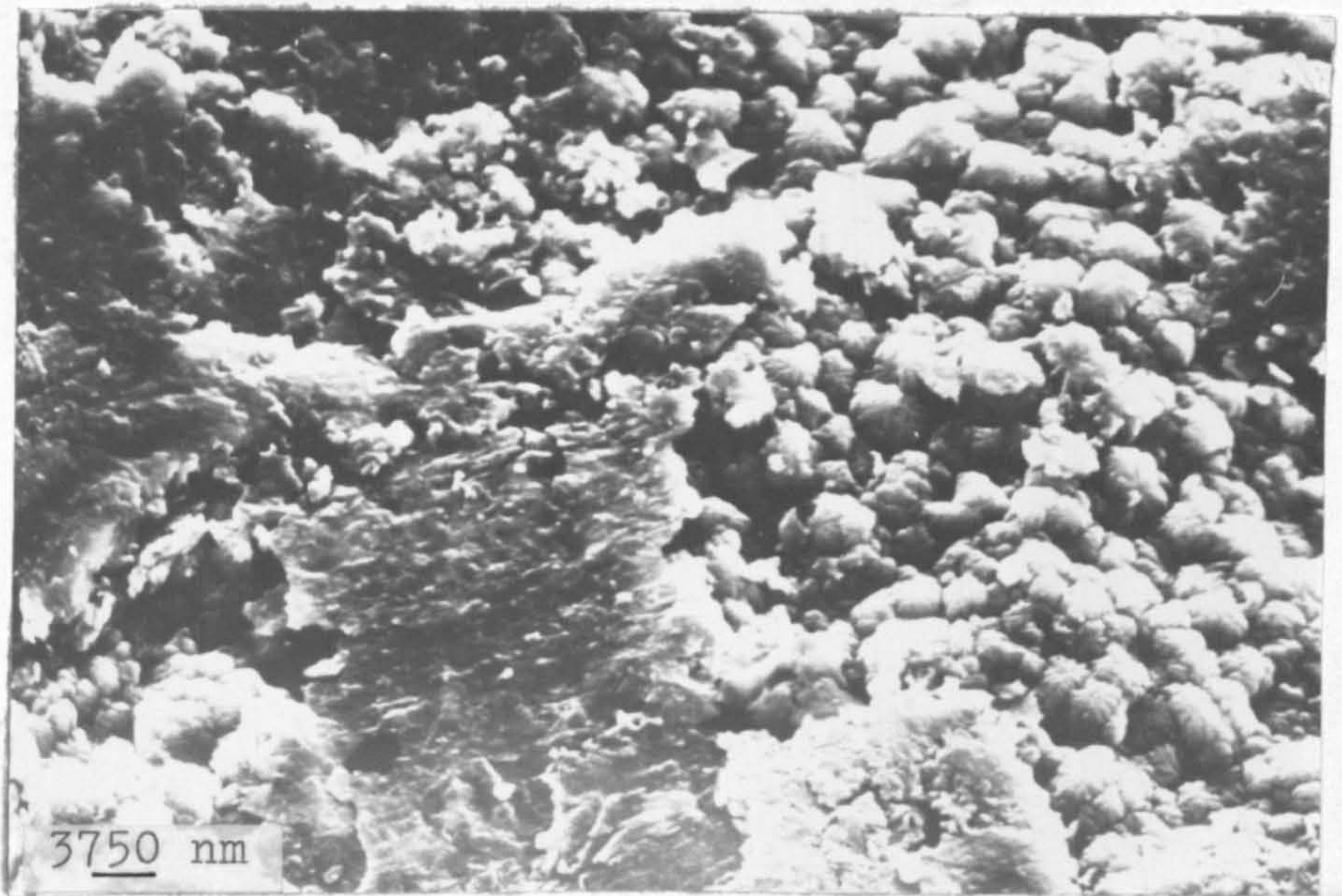
Fig.82. SEM showing the oxide/atmosphere interface of a sample which has been tested in a 'two-stage' experiment.
