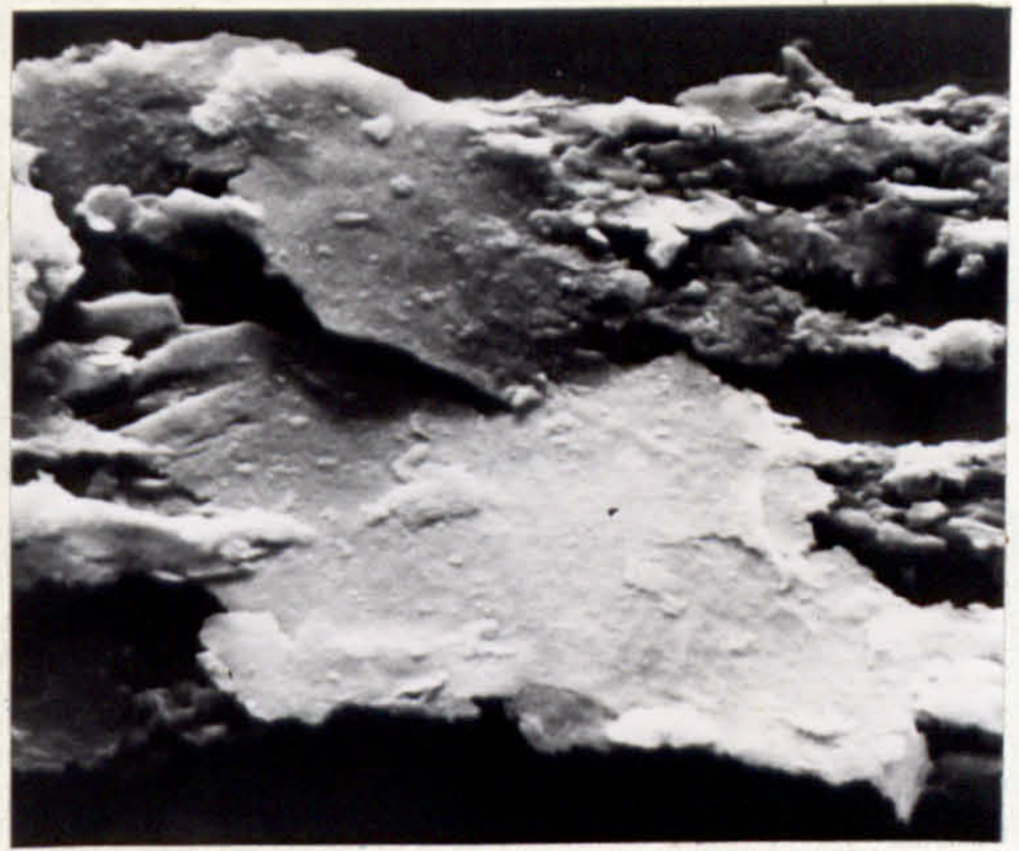
b) WEAR DEBRIS, BASE OIL 5 MINUTES.
