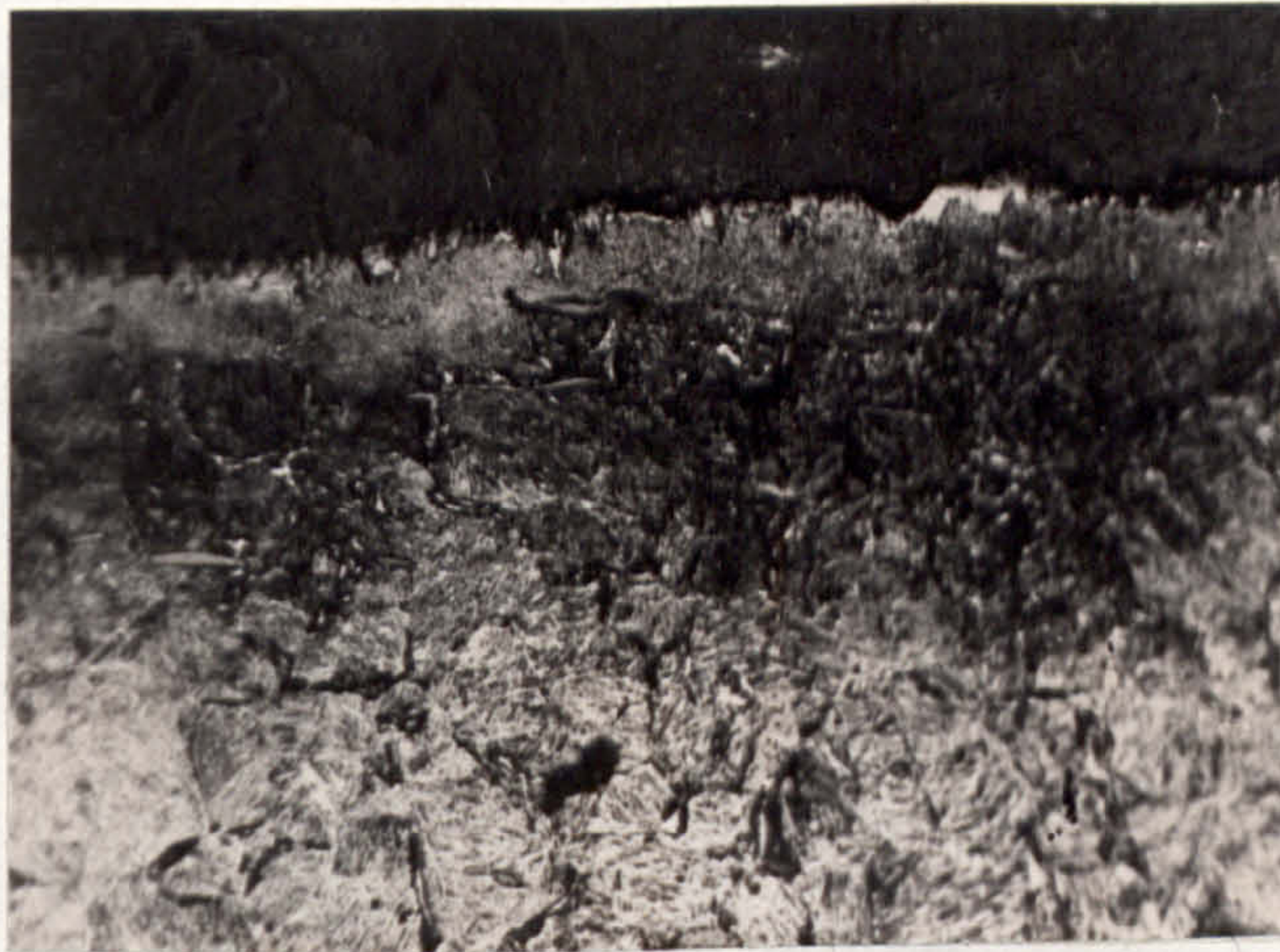
FIG. 48. TEST 1C, CAM SPECIMEN TAPERSECTION.
