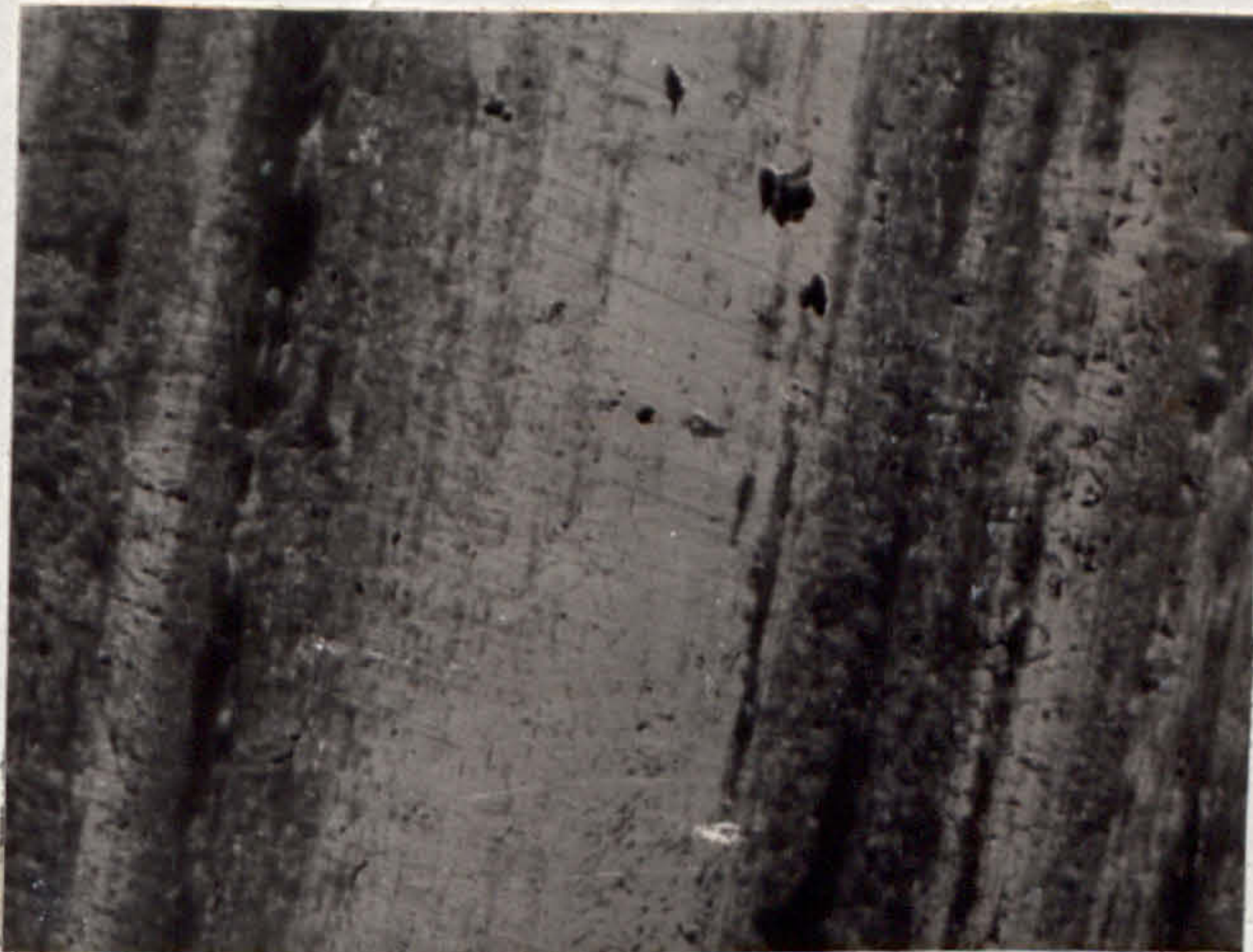
FIG. 38. TEST 1B, FOLLOWER WEAR SURFACE, ELECTRON MICROGRAPH.
