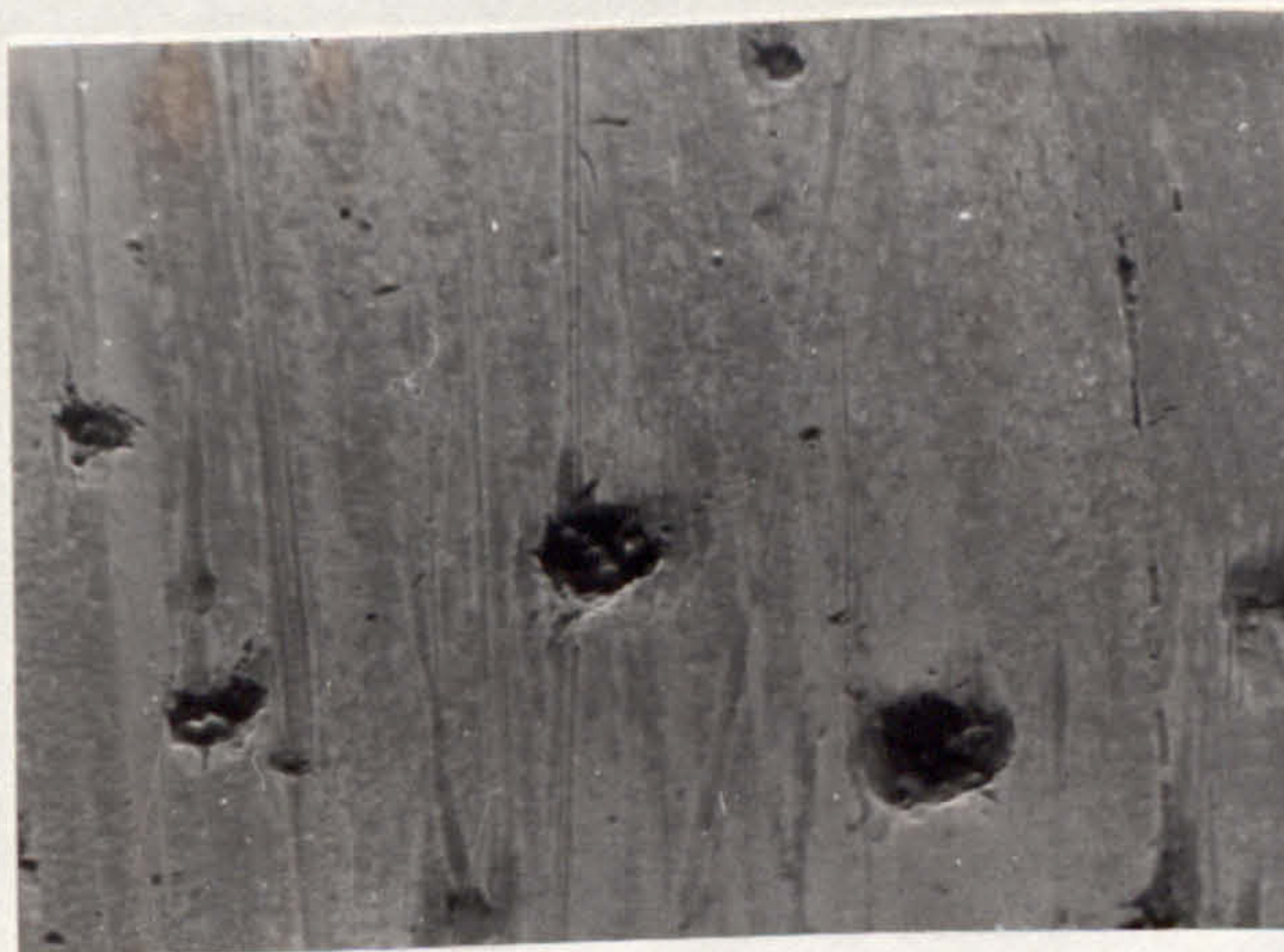
FIG. 87. TEST II, FOLLOWER WEAR SURFACE, ELECTRON MICROGRAPH.
