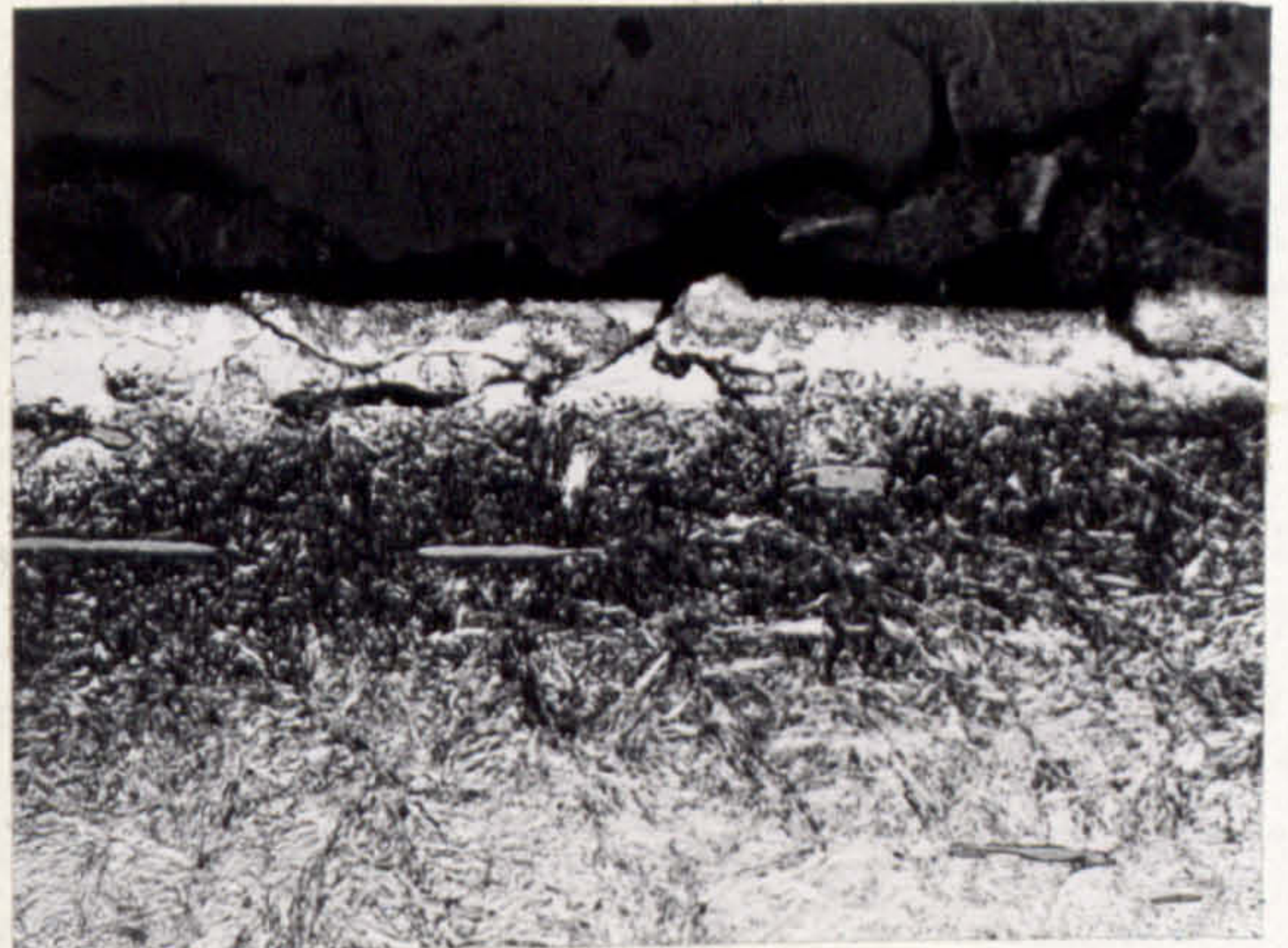
b) CAM TAPERSECTION, BASE OIL. 1 HOUR.
