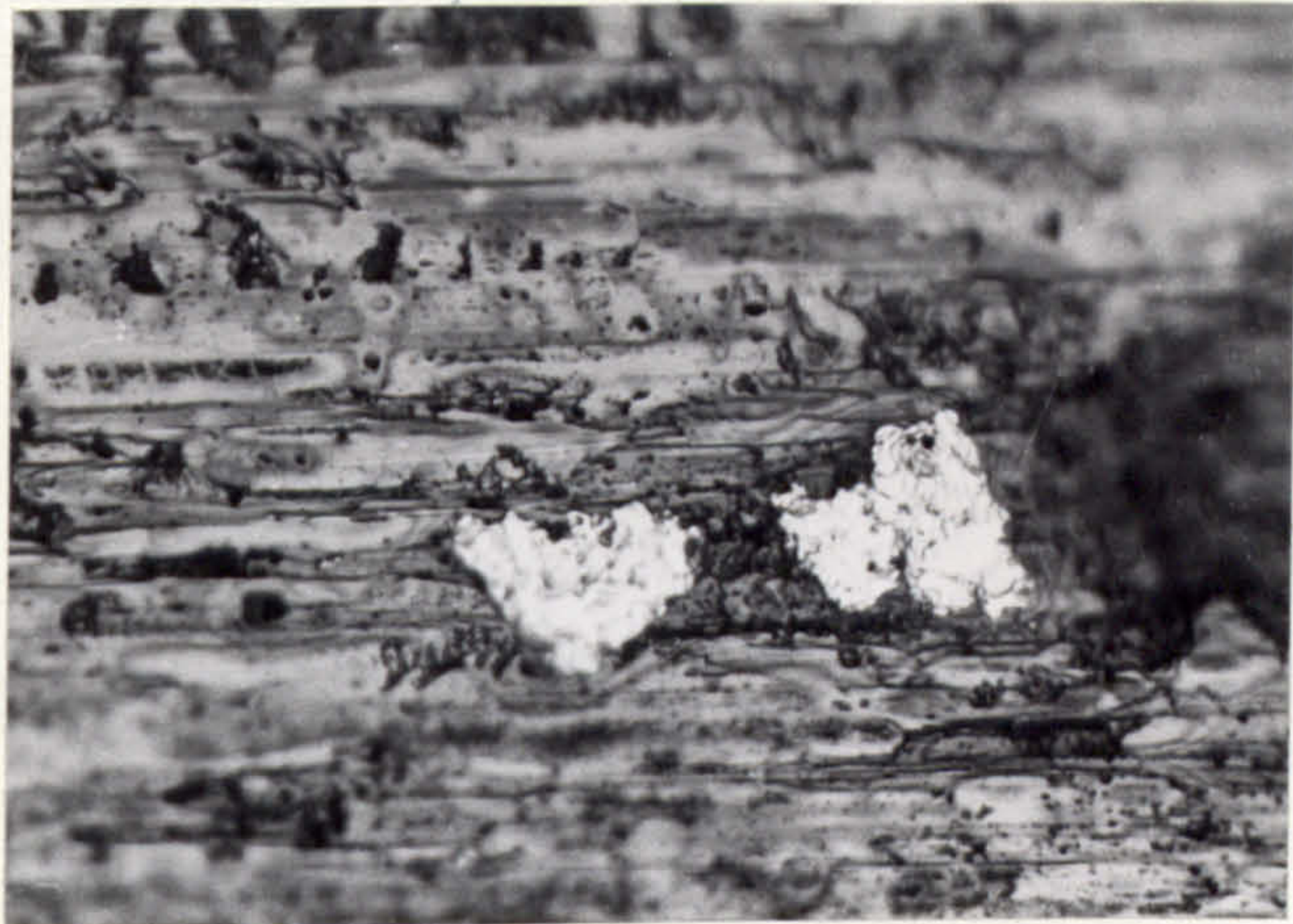
FIG. 176. TEST 3G, CAM WEAR SURFACE, OPTICAL.
