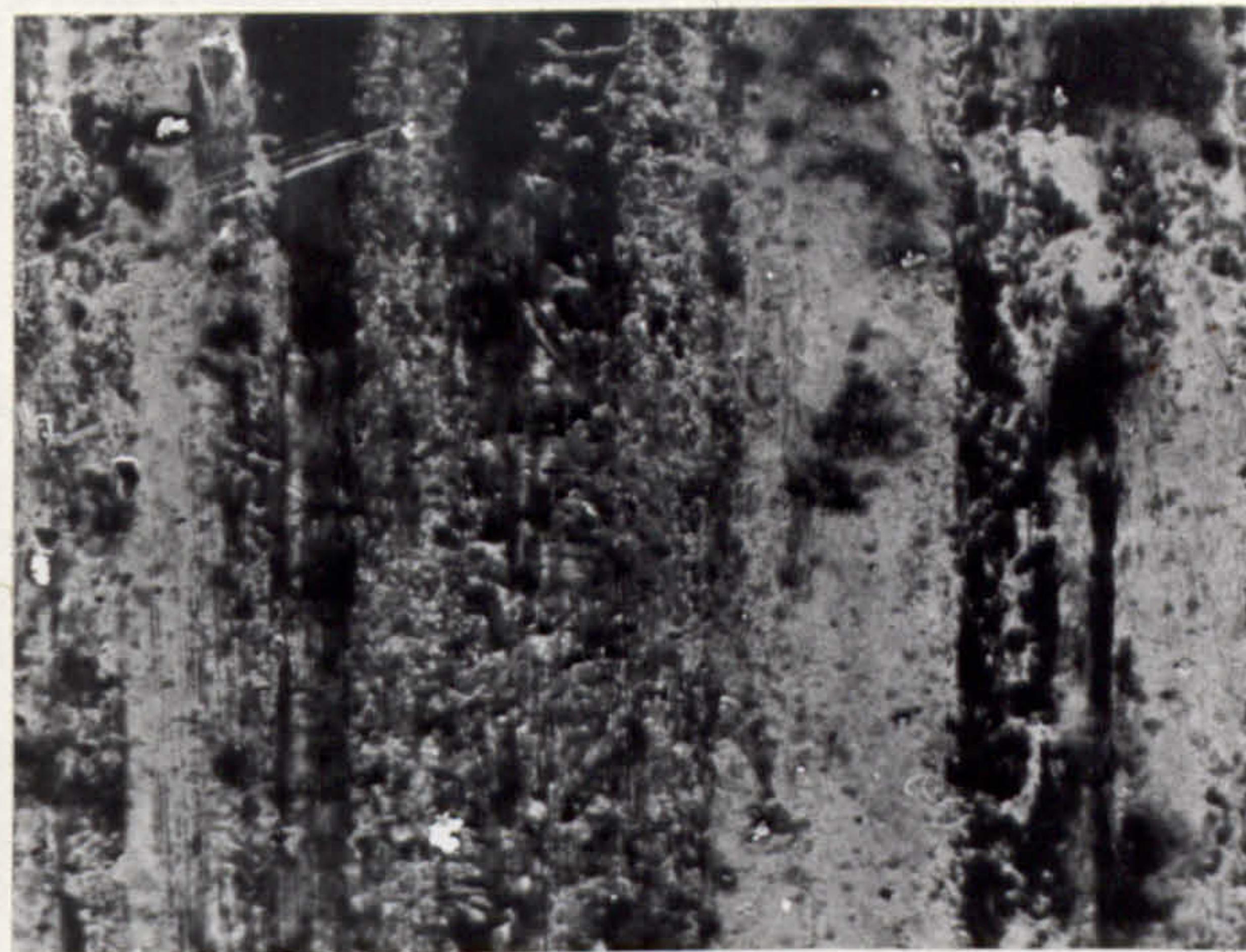
FIG. 135. TEST 20 - ELECTRON MICROGRAPH FOLLOWER WEAR SURFACE, 50 HOURS.
