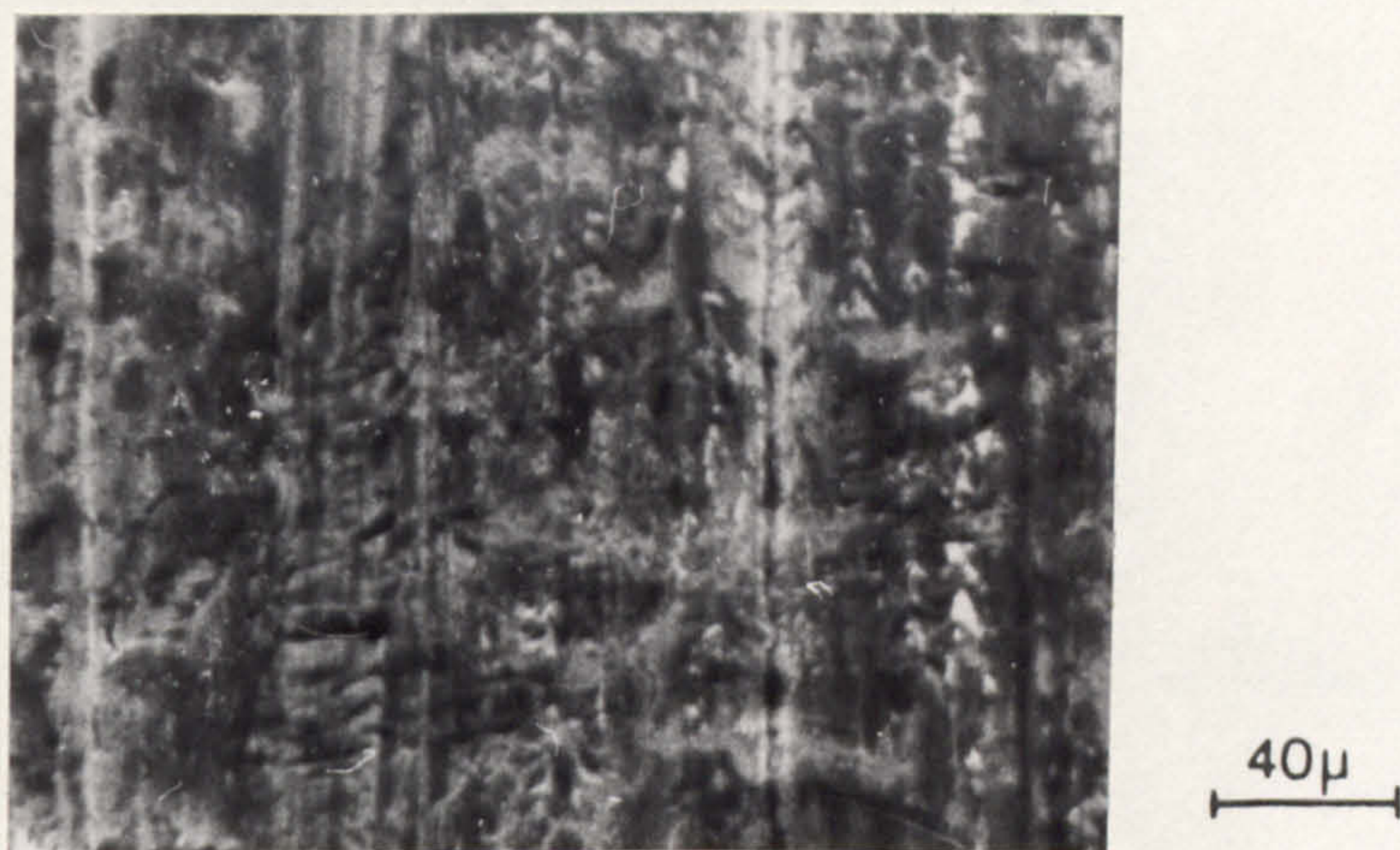
FIG. 139. TEST 2D - ELECTRON MICROGRAPH FOLLOWER WEAR SURFACE, 70 HOURS.
