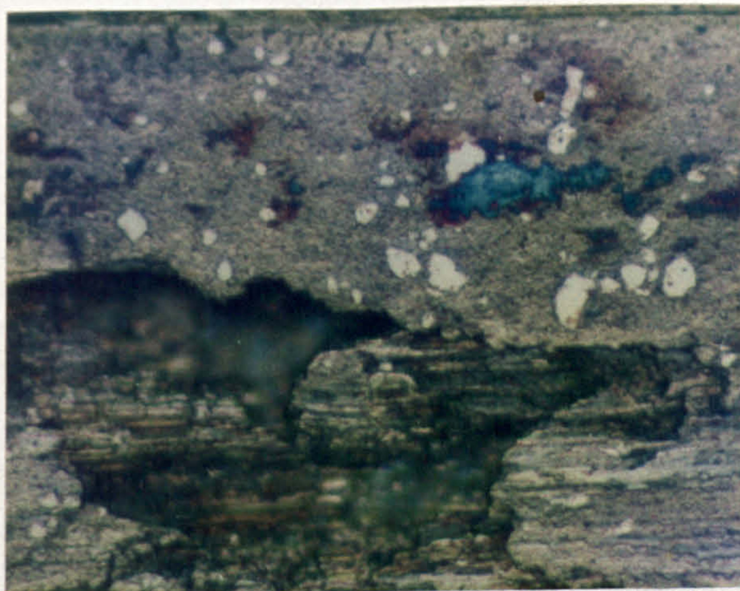
FIG. 34, TEST 1B, CAM WEAR SURFACE. OPTICAL.
