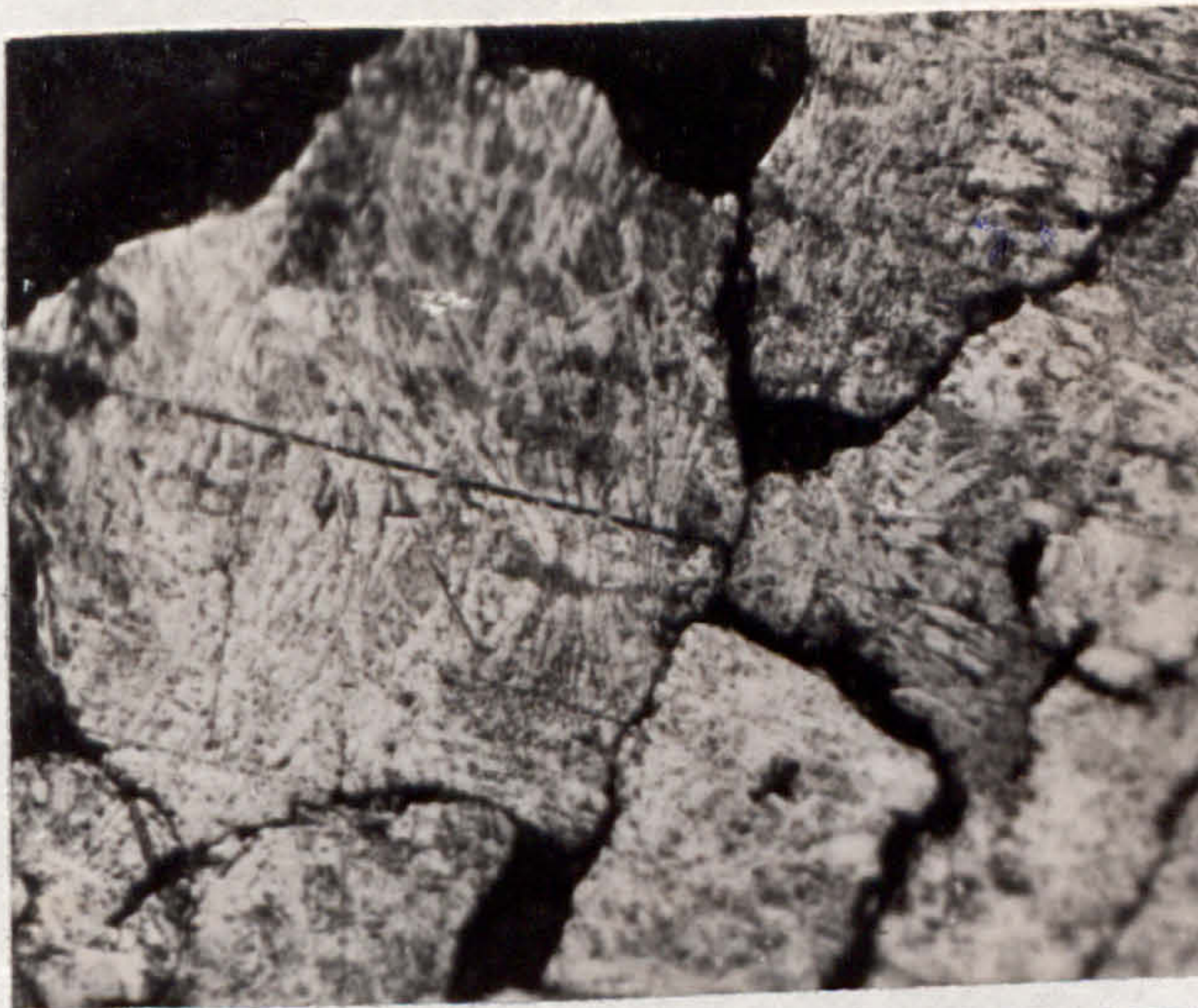
FIG. 45, TEST 1C, FOLLOWER WEAR SURFACE, OPTICAL.
