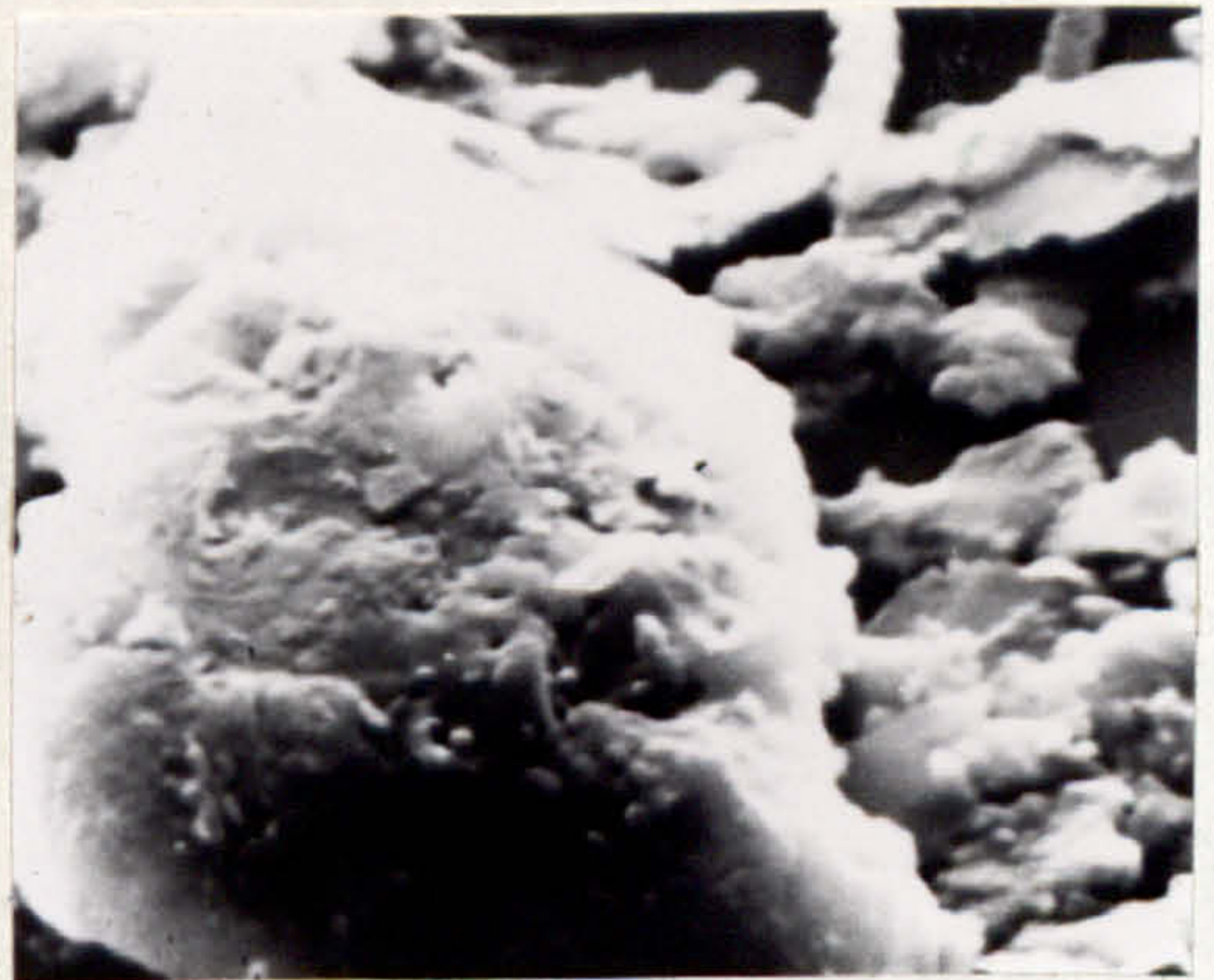
d) WEAR DEBRIS, BASE OIL 50 HOURS
