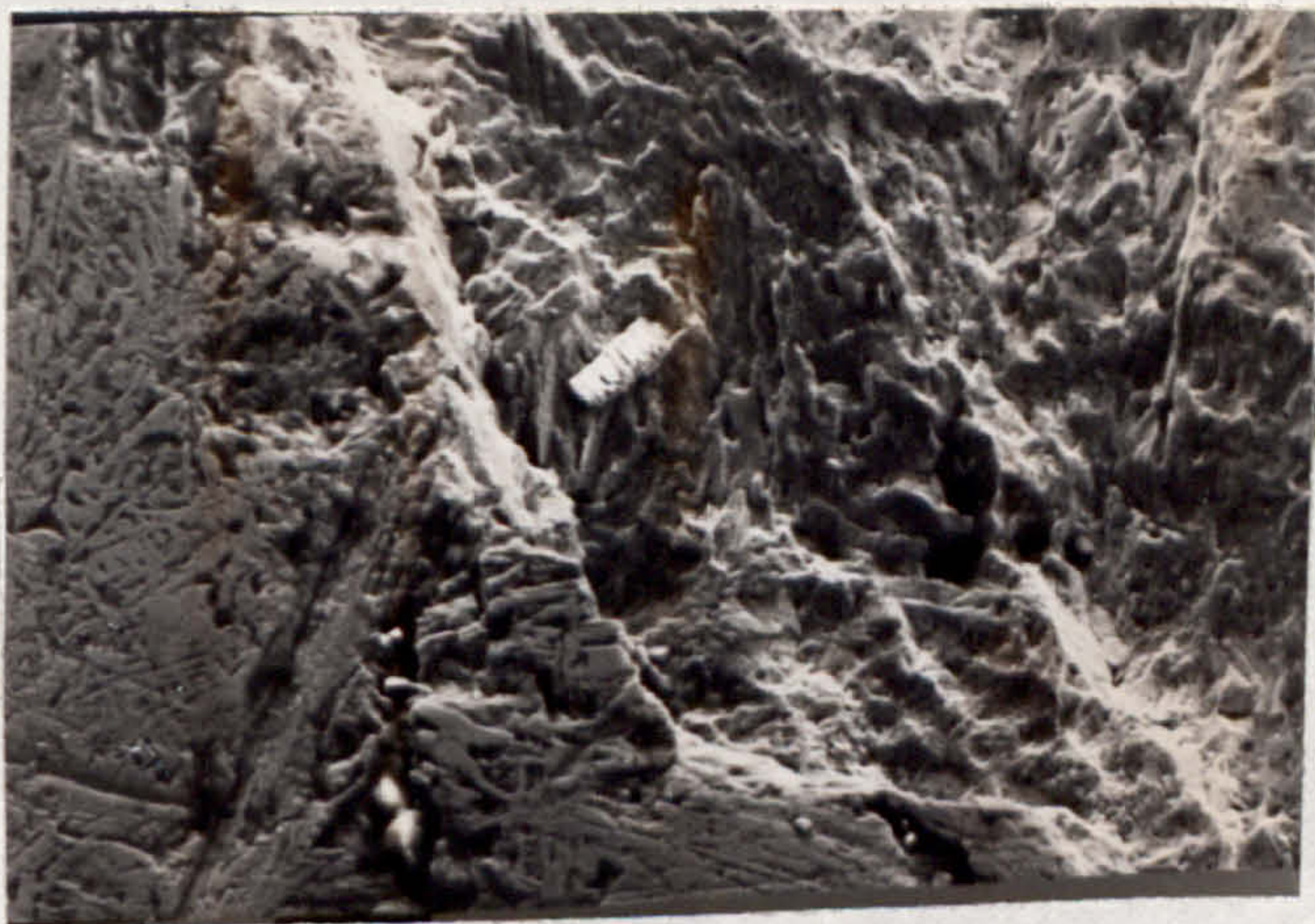
FIG. 47, TEST 1C, FOLLOWER WEAR SURFACE ELECTRON MICROGRAPH.
