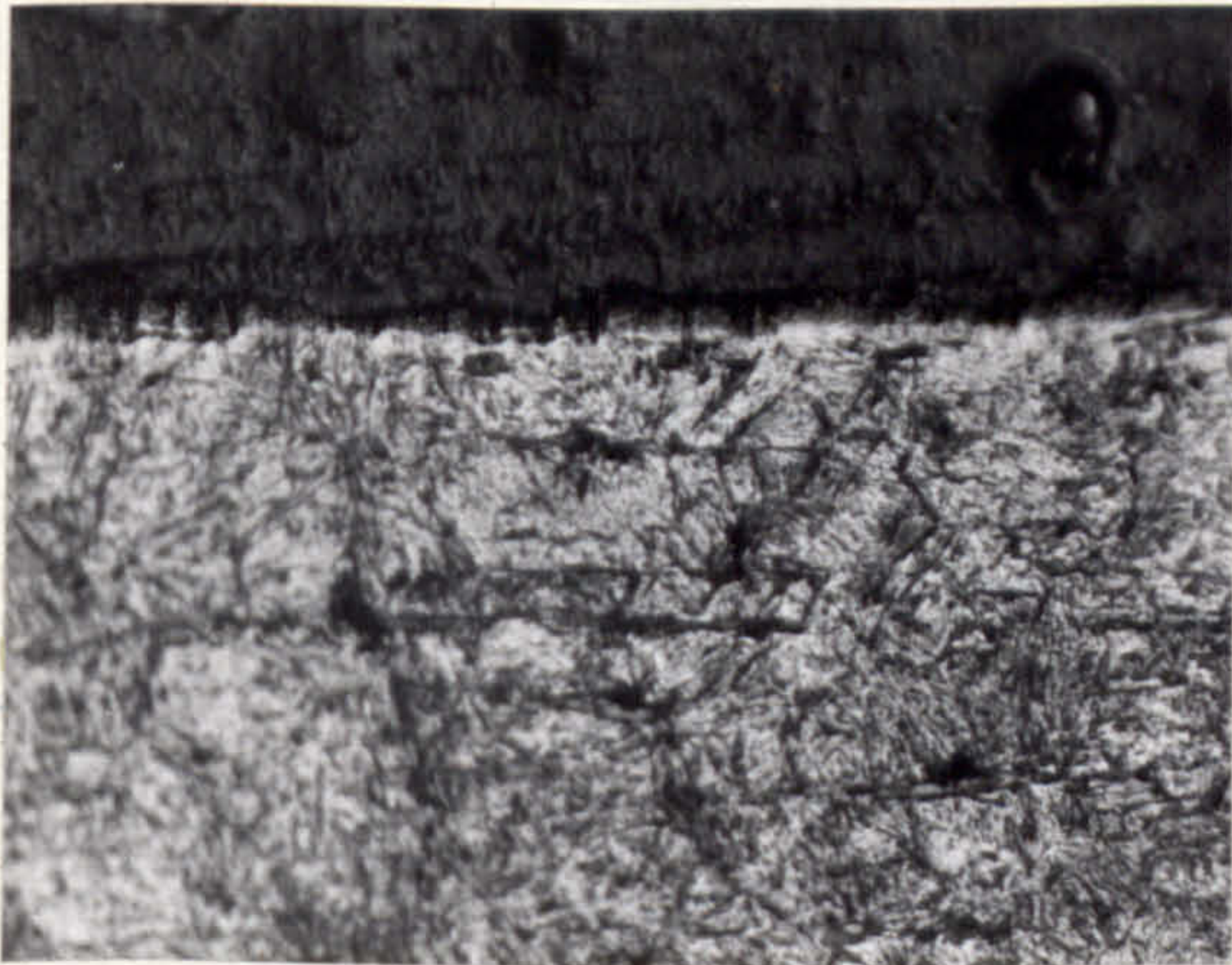
a) CAM TAPERSECTION, FULLY FORMULATED OIL. 75 HOURS
