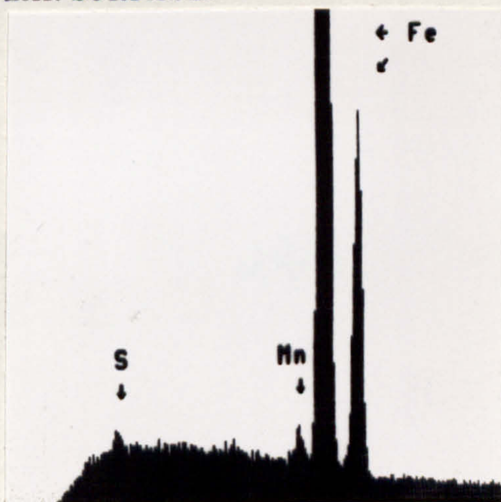
FIG. 146. TEST 2E - X-RAY ENERGY SPECTRA CAM WEAR SURFACE.
