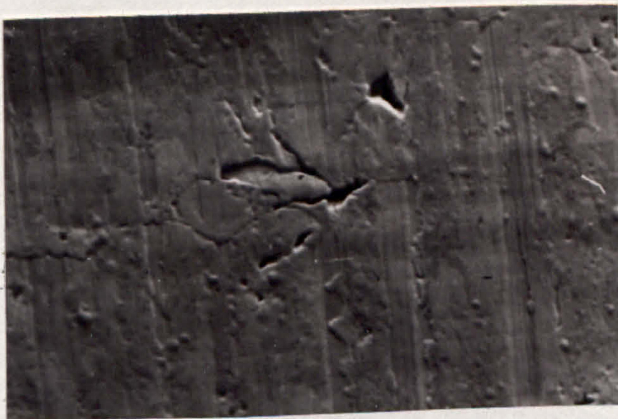
FIG. 69. TEST 1F, FOLLOWER WEAR SURFACE, ELECTRON MICROGRAPH.
