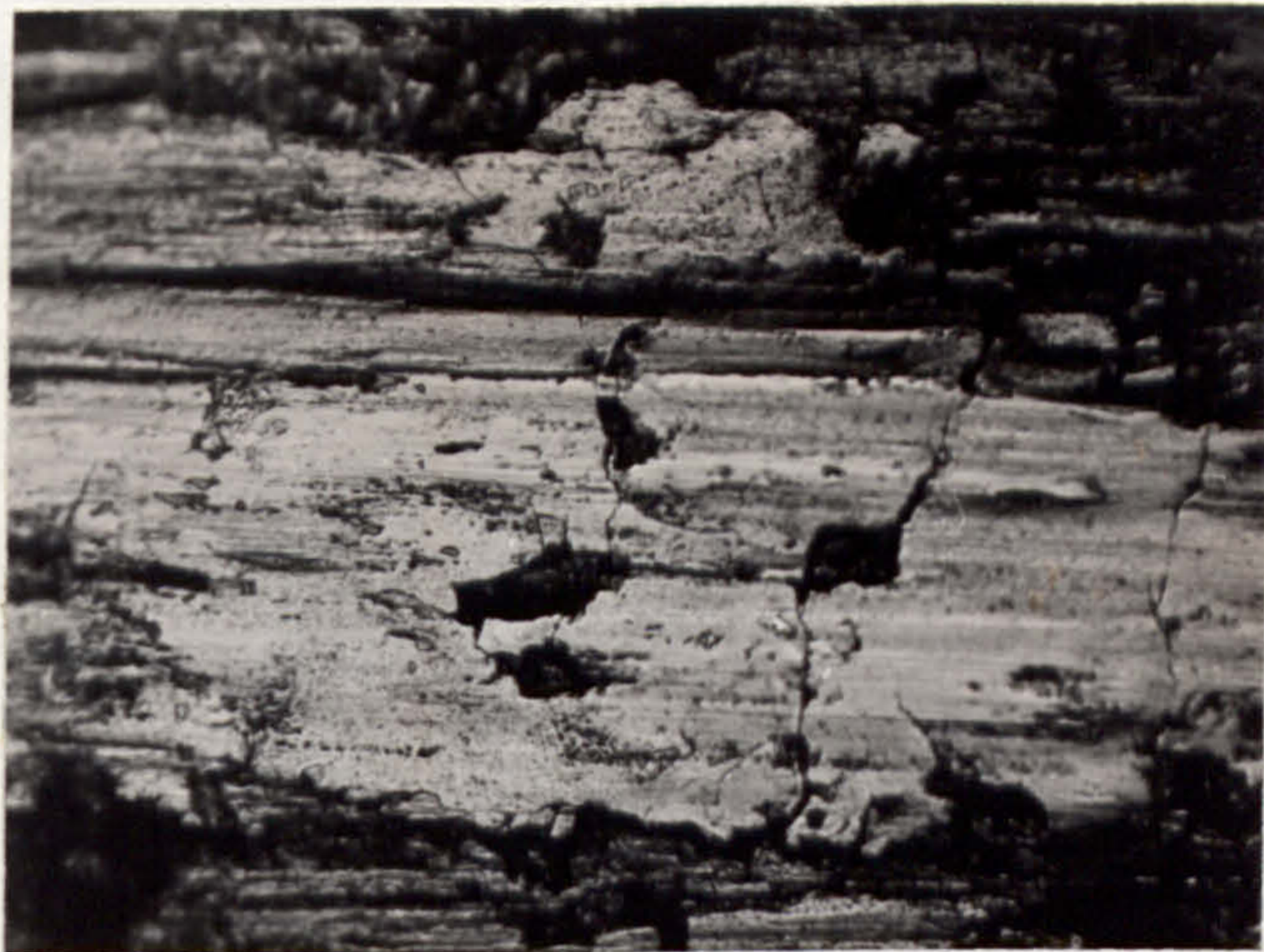
FIG. 103. TEST 1L, CAM WEAR SURFACE, OPTICAL.
