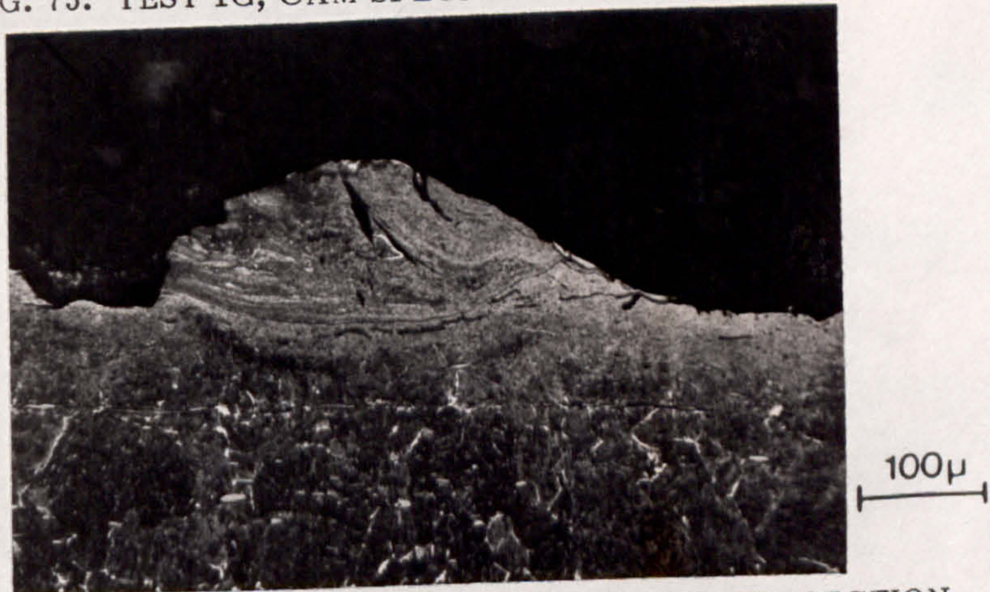
FIG. 76. TEST 1G, FOLLOWER SPECIMEN TAPERSECTION.
