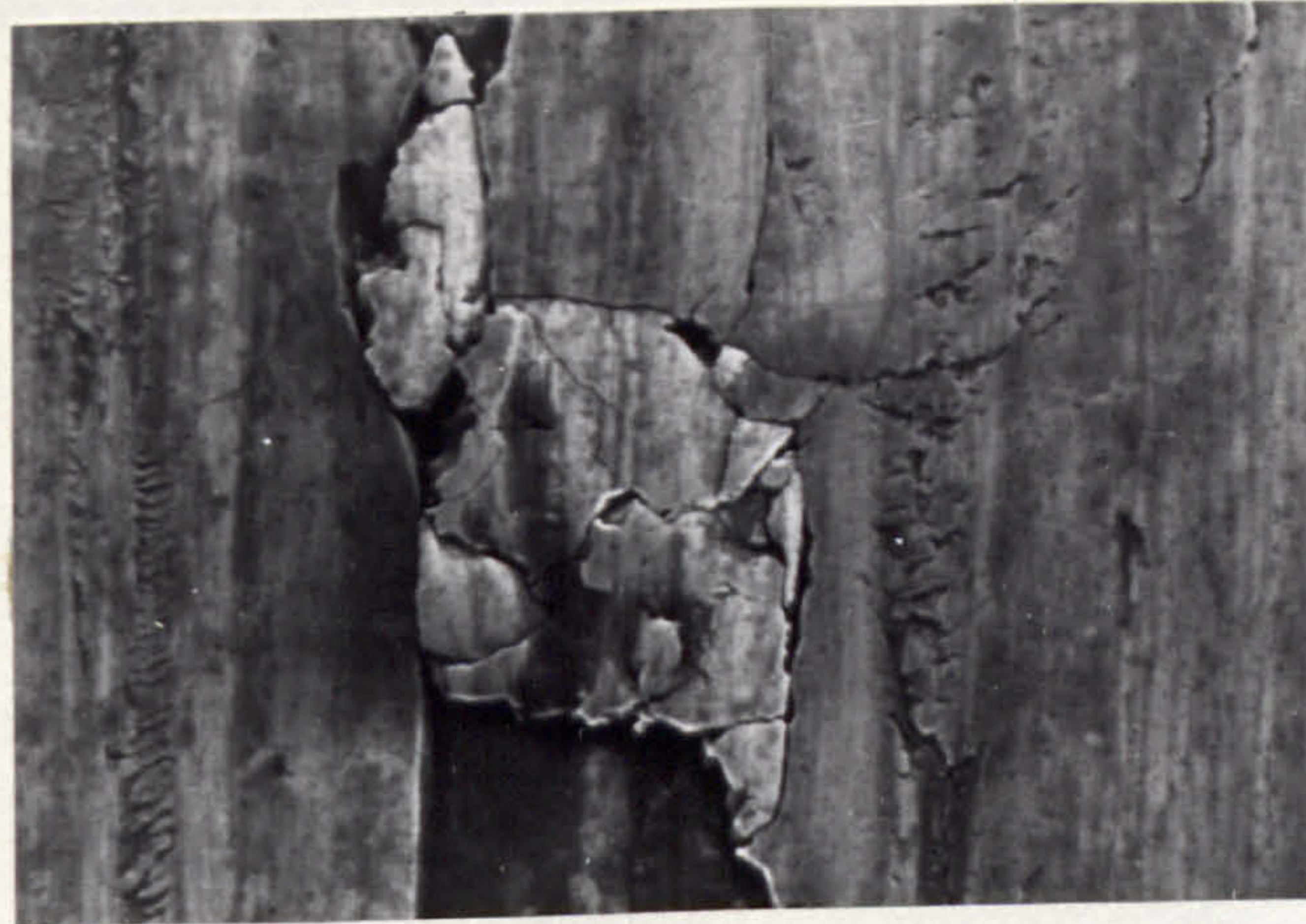
FIG. 163. TEST 3E, CAM WEAR SURFACE ELECTRON MICROGRAPH.
