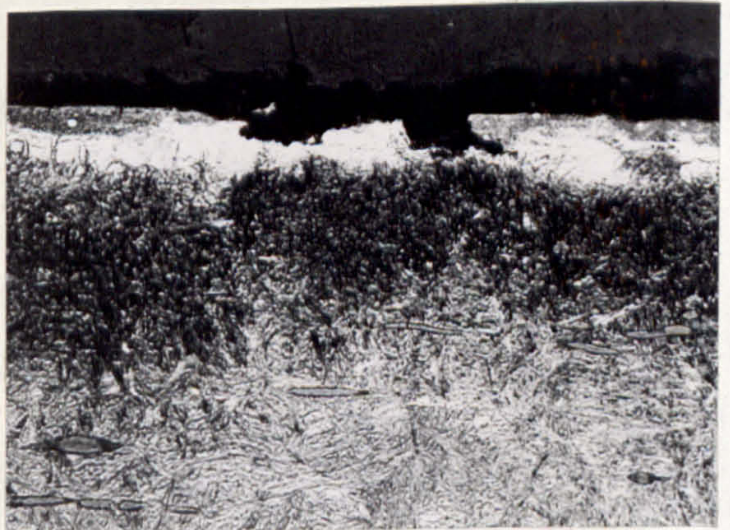
c) CAM TAPERSECTION, BASE OIL. 75 HOURS.
