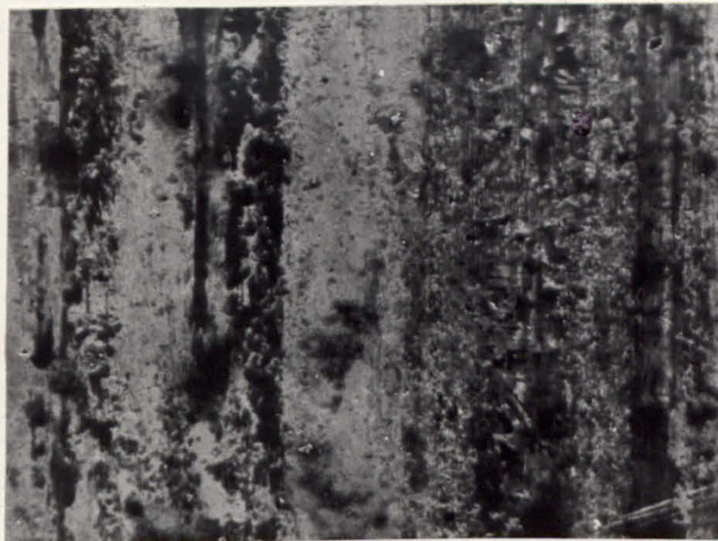
FIG. 137. TEST 2D - ELECTRON MICROGRAPH, FOLLOWER WEAR SURFACE, 60 HOURS.
