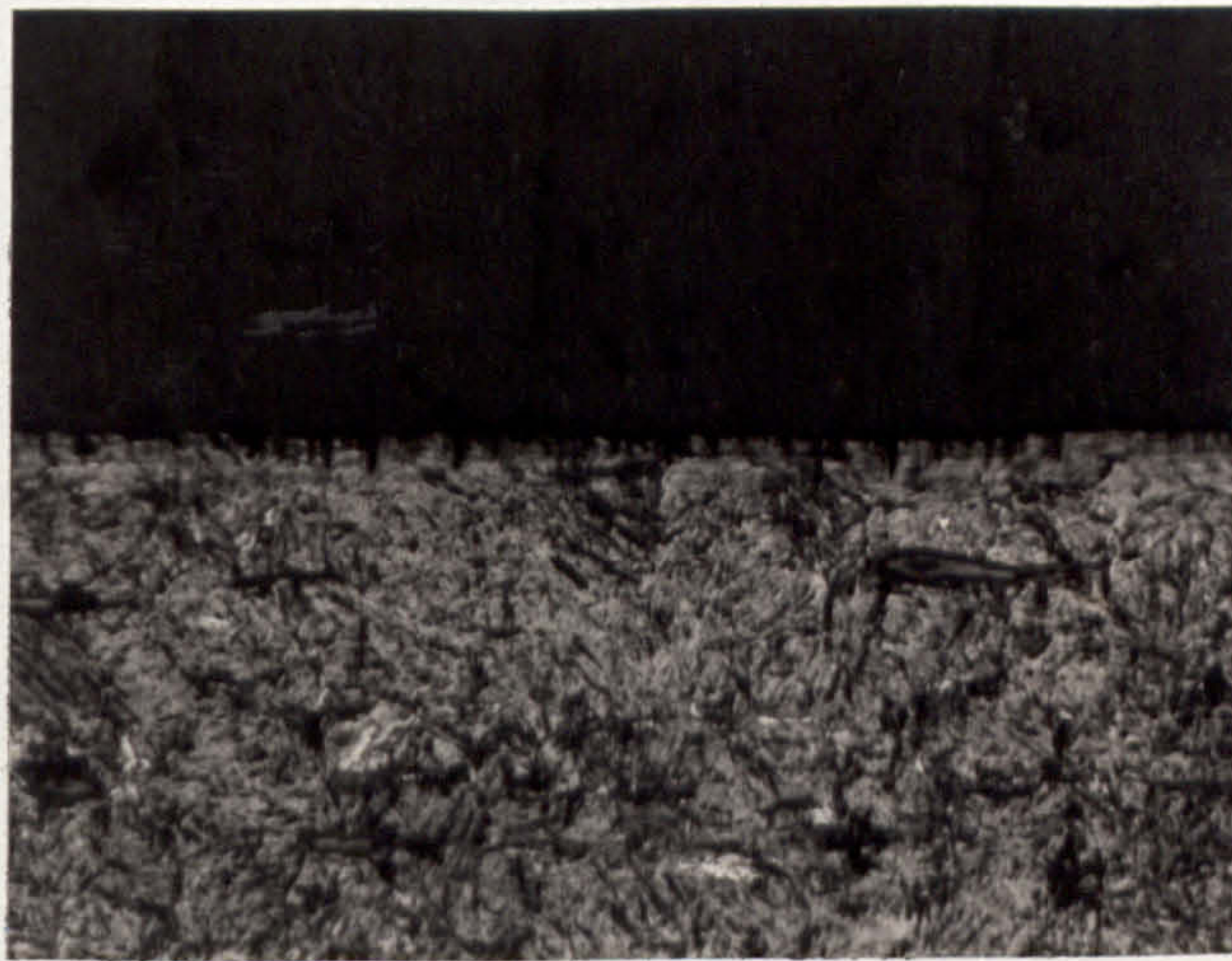
FIG. 31, TEST 1A, CAM SPECIMEN TAPER SECTION.
