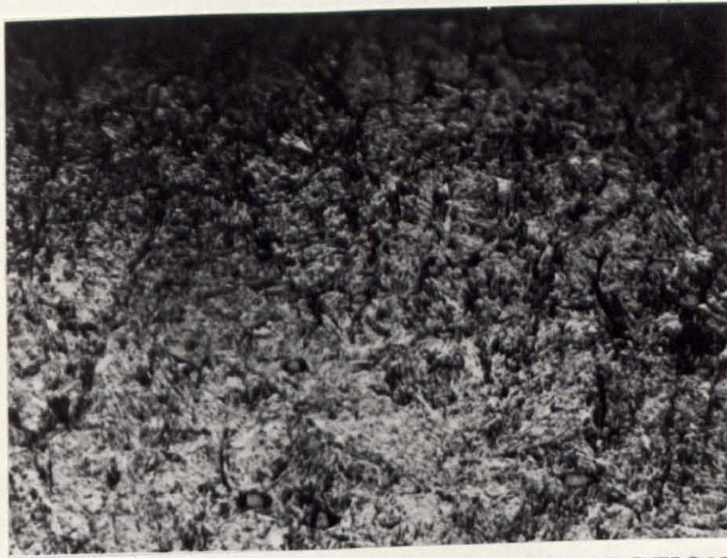
FIG. 130. TEST 2C - CAM SPECIMEN TAPERSECTION.
