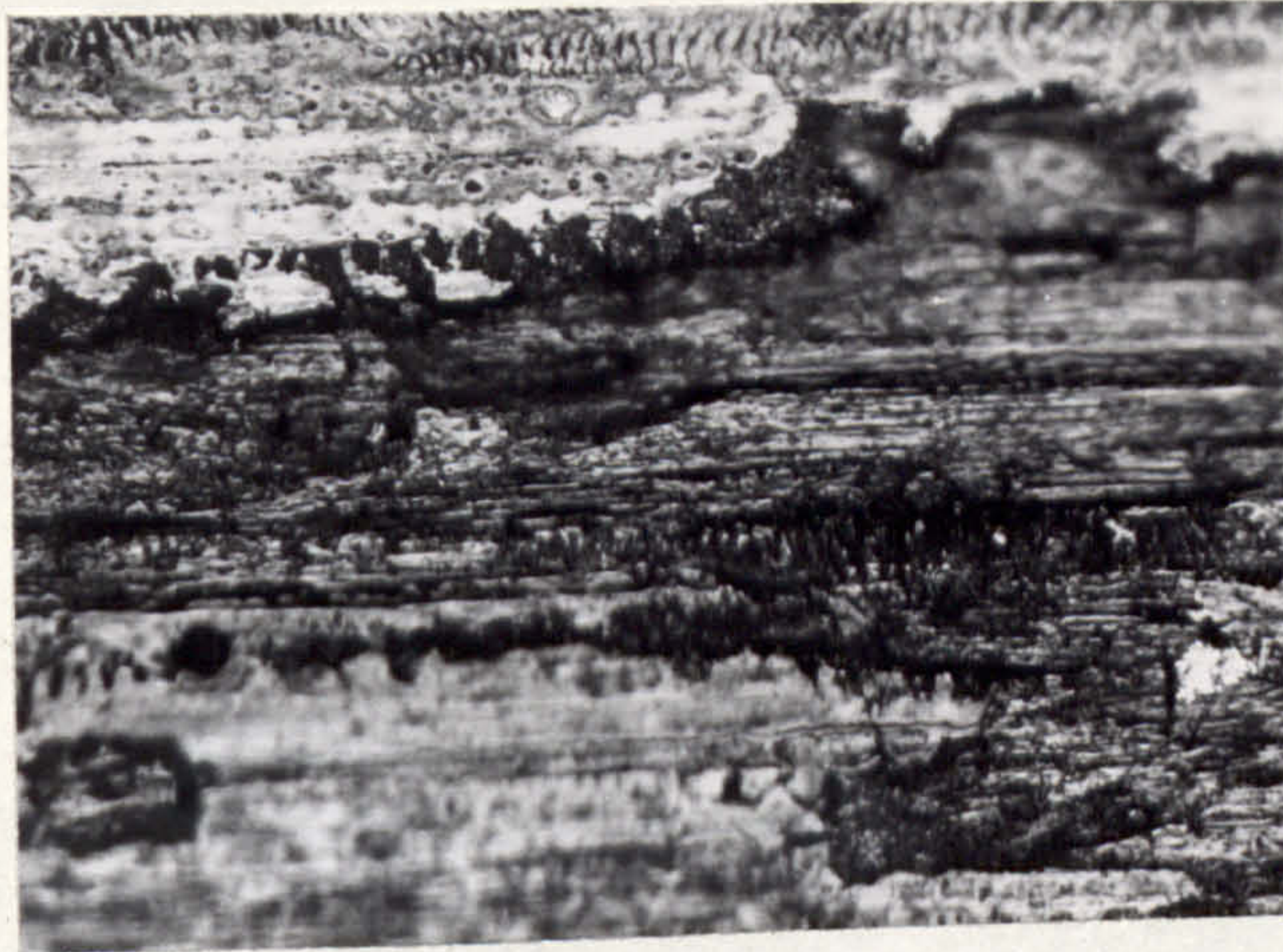
FIG. 161. TEST 3E, CAM WEAR SURFACE, OPTICAL.
