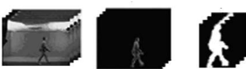
Fig 1.4 Image sequence-background subtraction-image binarisation and normalization (Lam et al. 2007).
