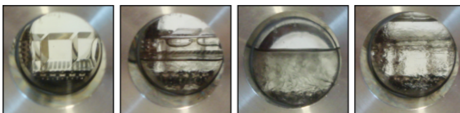
Figure 4.8 Liquid CO 2 entering autoclave (photos taken at 0-30 minutes into drying).
