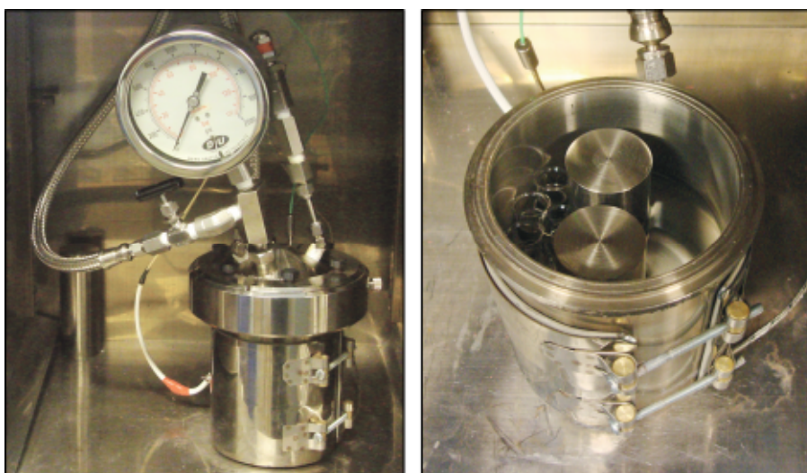
Figure 4.4 Closed HTSCD autoclave (left), view inside autoclave (right).
