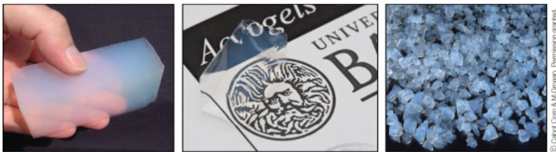
Figure 2.21 Translucent monolithic aerogel (left), transparent monolithic aerogel (centre), and translucent aerogel granules (right).
