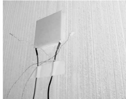
Above: Close-up photograph of the peltier module and two thermocouples mounted to the 10mm thick aerogel panel.
