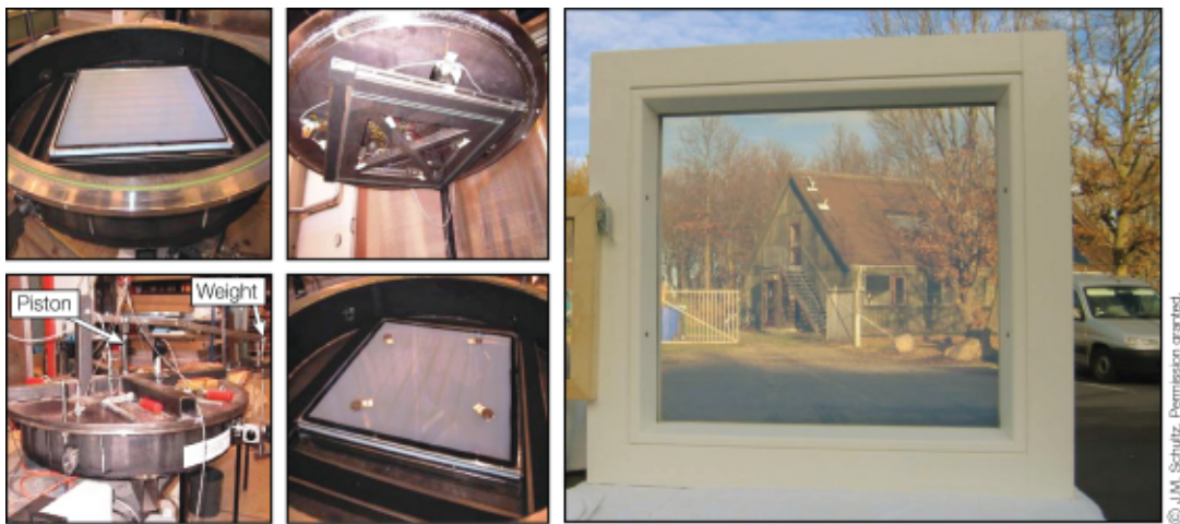
Figure 2.29 Aerogel glazing prototypes produced by Schultz and Jensen (2008).
