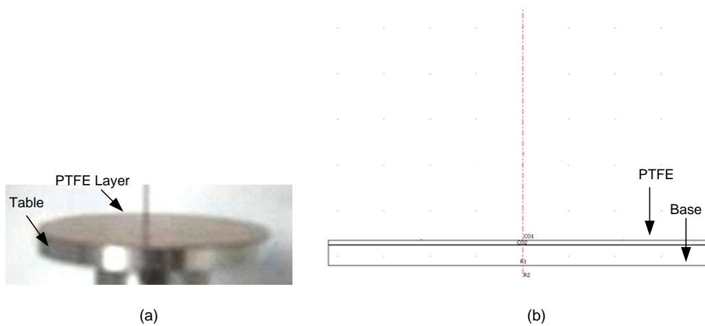
Figure 4.12 a) Shape of table in experimental setup b) Geometry of table in COMSOL
