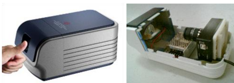
Figure 3.6: Optical Device for high resolution fingerprint imaging [128]
