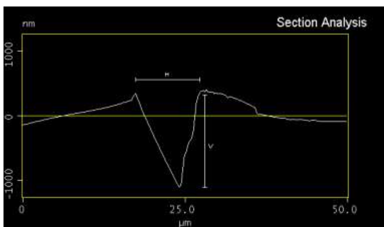
Figure 4.2 – A representative cross-sectional view of one area from one scratch on the donor A sample substrate. Slopes either side of the scratch opening, caused by physical stresses during scratching, are clearly evident.
