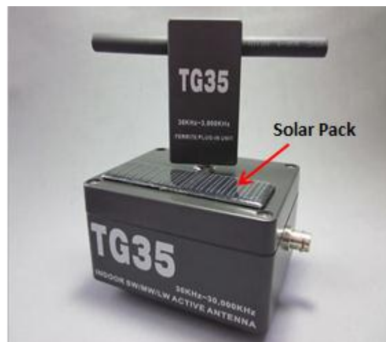
Figure 7.1 The TG35 self-powered radio antenna uses a solar pack to harvest energy to power it [6].
