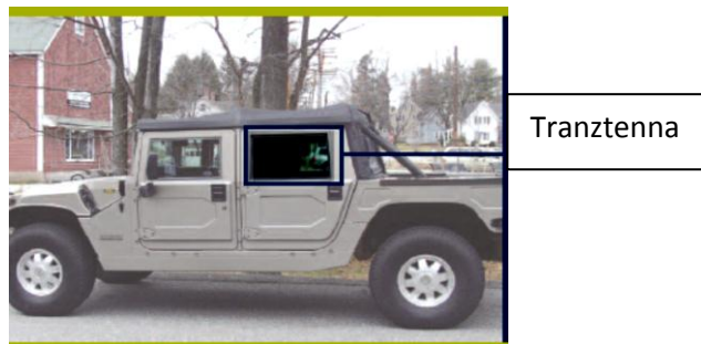
Figure 2.17 The Tranzenna mounted on the side window of a military jeep [4].
