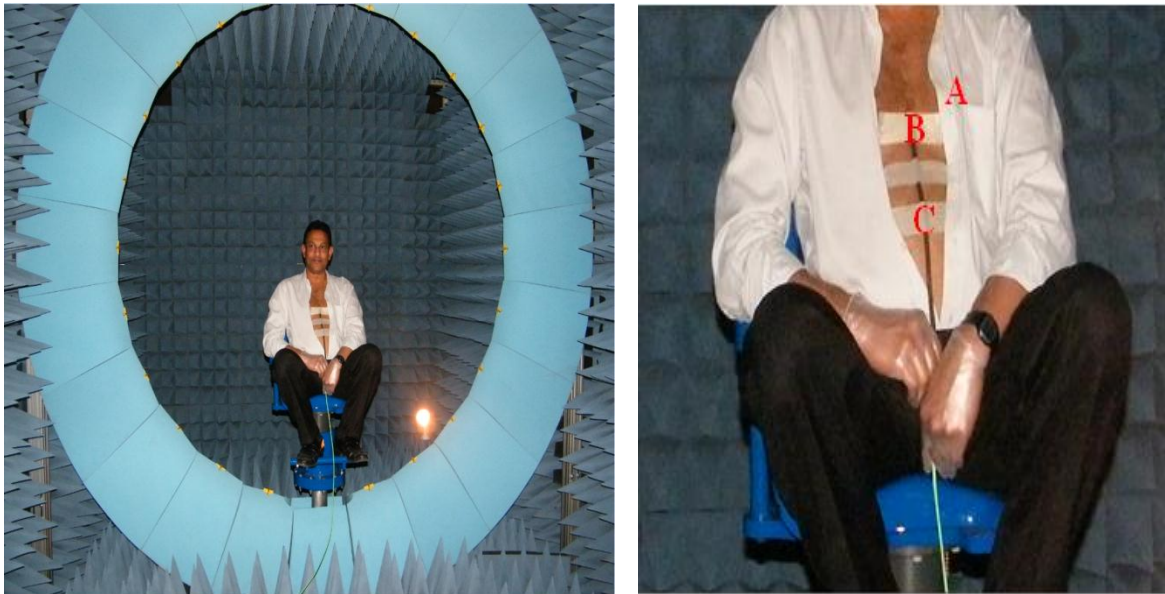
Figure 5.2 Measurement set-up in the anechoic chamber for the heart (a), chest (b), and belly (c) on-body area tests.
