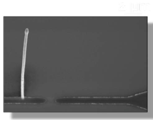
Figure 9. A vertical gold nanowire on an electrode, from Ref. [10].
