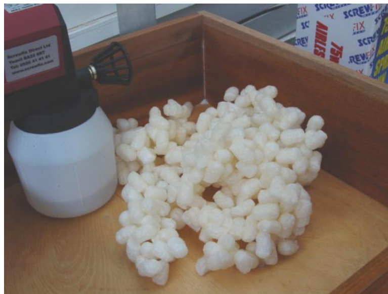
Figure 3.9: Manual wetting of loosefill chips showing immediate adhesion at contact points
