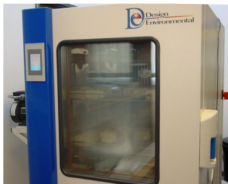
Figure 4.8: Samples during conditioning in the Delta 190-40HS conditioning chamber
