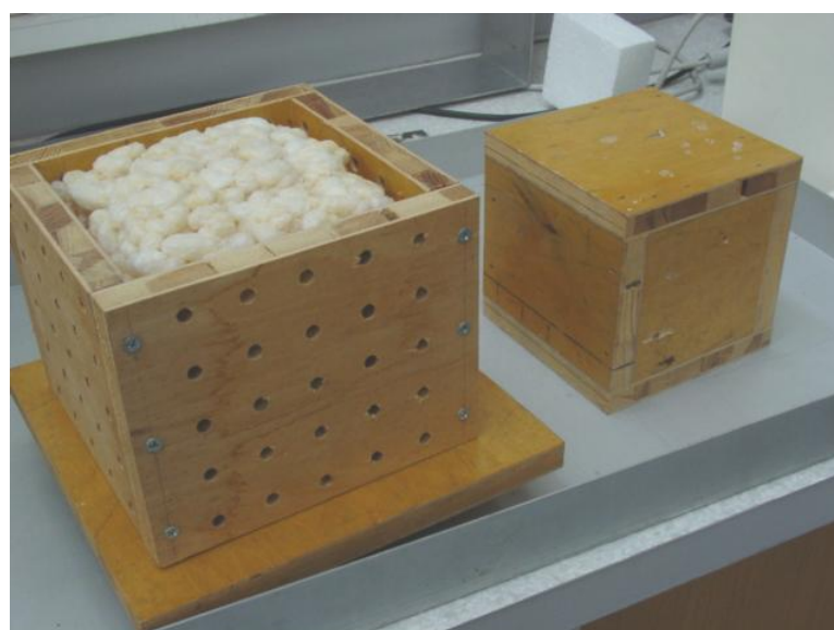
Figure 3.10: Set-up for compression of the moistened loosefill
