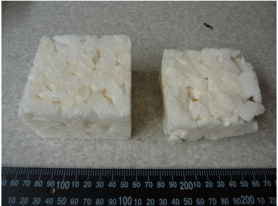
Figure 4.10: Non-uniform shrinkage of CBL sample subjected to high temperature and high humidity conditioning (right), alongside an untreated sample (Sample densities approx. 46 \text{ Kg/m}^3 . Post-conditioned sample density 73 \text{ Kg/m}^3 )
