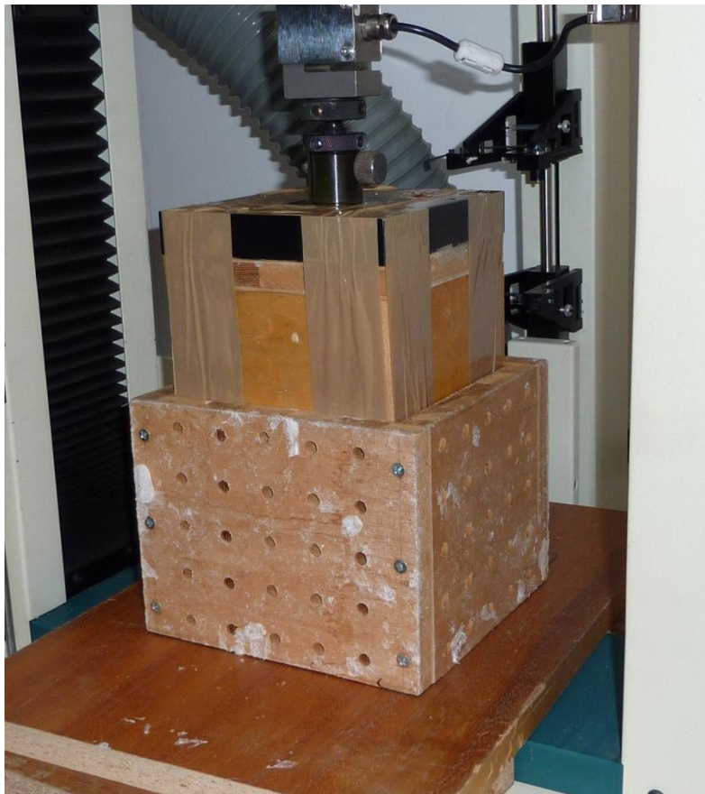
Figure 4.1: CBL sample being produced on the Hounsfield testing machine
