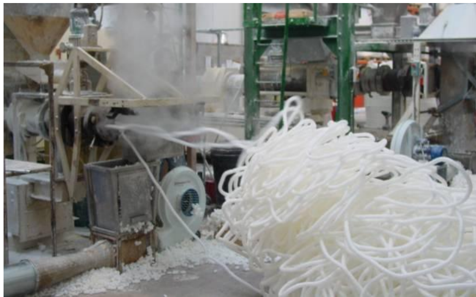
Figure 3.1: Continuous starch foam strands being extruded (rotating cutter removed)
