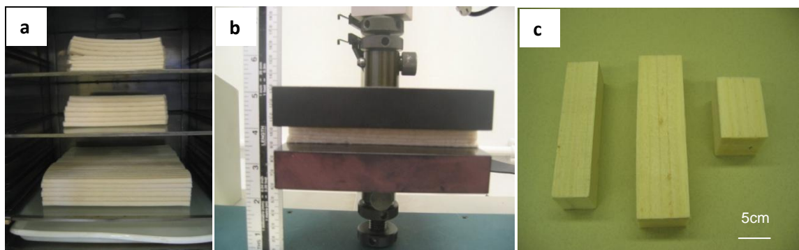
Figures 4.19 a), b) & c): Preparation of high-density RPS block foam samples utilising high-humidity conditioning and compression (Wang, 2008)
