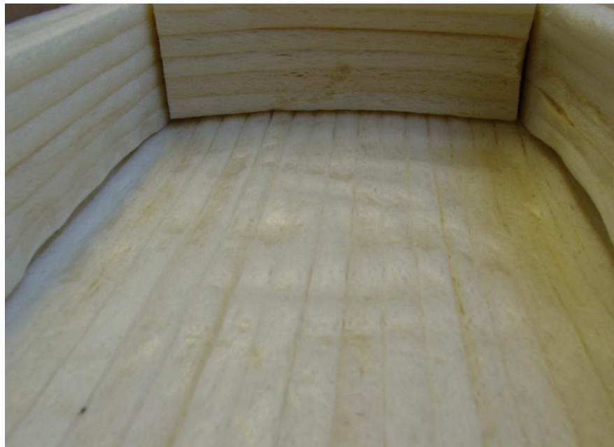
Figure 6.14: Slight deformation of the unlined RPS foam following the second transit trial
