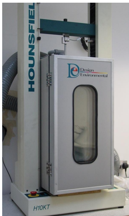
Figure 4.9: Hounsfield mechanical testing machine fitted with Design Environmental auxiliary testing chamber
