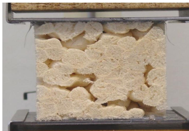
Figure 4.7: CBL sample undergoing a tensile test
