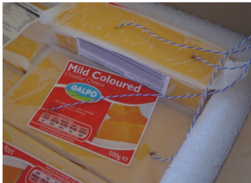
Figure 4.23: Thermocouple positions within the PE foam-lined coolbox (prior to sealing)
