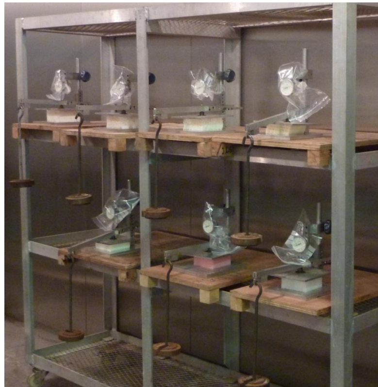
Figure 4.14: Samples undergoing creep tests in the Climatec tropical chamber at Pira International Ltd.
