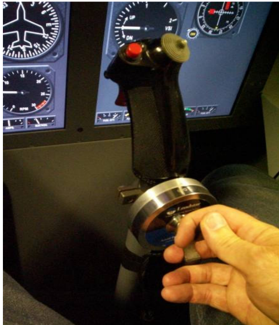
Figure A4-3, Digital Load Cell used for Calibration of the Stick Force Gradient
