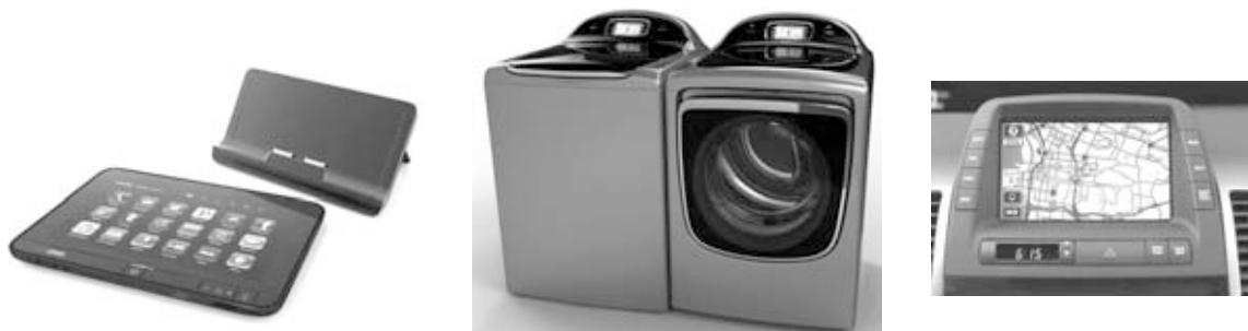
Figure 18: One Peak tablet to control smart appliances using proprietary OS and hardware developed by Whirlpool. Also showing Whirlpool Vantage smart appliance series and Toyota Prius navigation unit.
