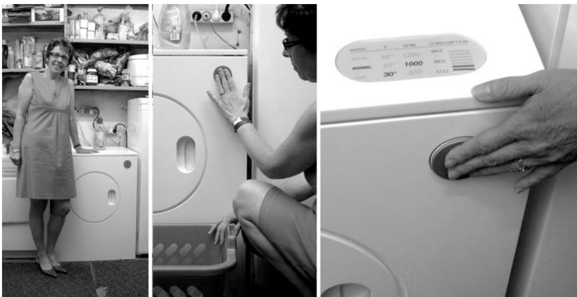
Figure 5. Joëlle H. is presenting OneWash, a washing machine with an interface mimicking the interface of a copy machine putting forward a large green button – in that case, for an ecological optimised programme – but still leaving the possibility to adjust the presets.
