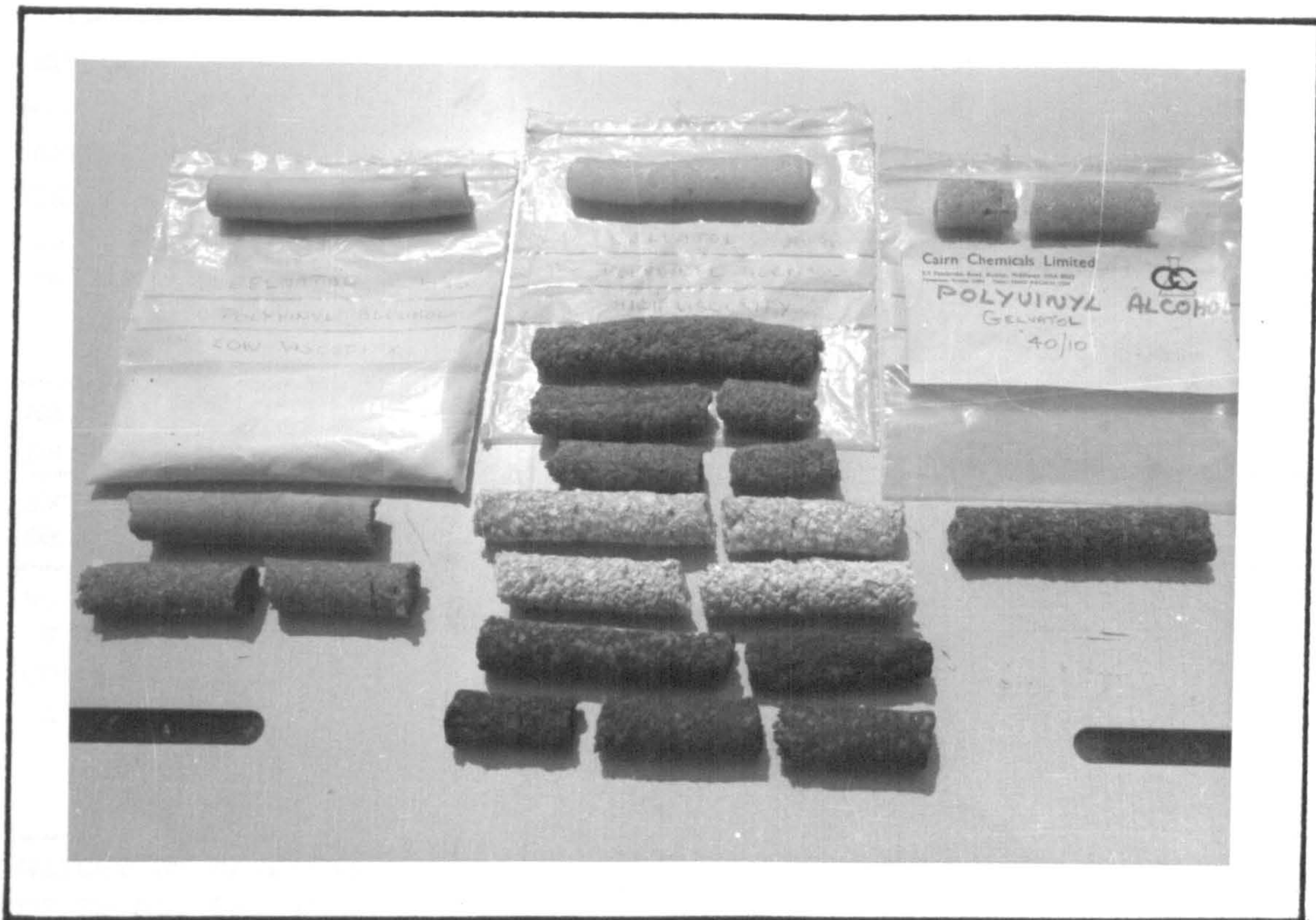
FIGURE 5/5. - A Variety of the Different 'Models' Produced From P.V.A. Powder, (With and Without 'Filler' Materials).
