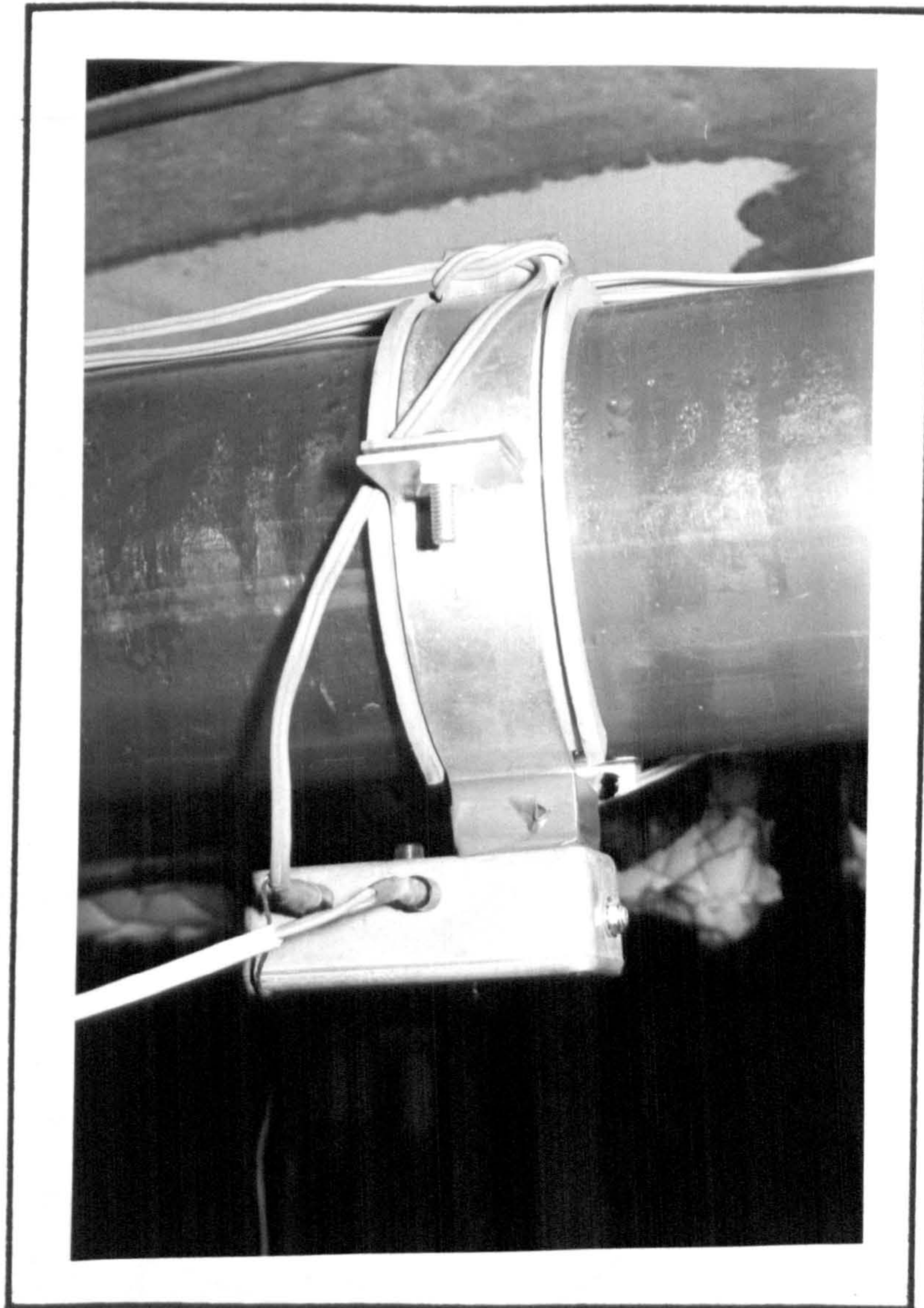
FIGURE 8/8. - Photo Cell / Light Source Arrangement, ('On-Site').
